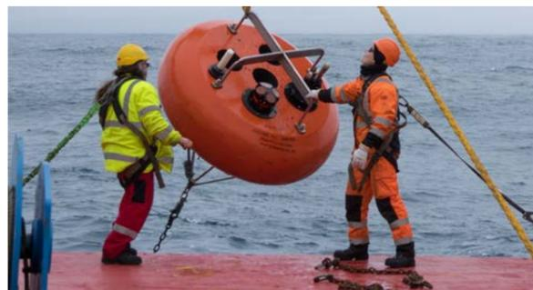
The passive acoustic device being collected off SGSSI (Credit: British Antarctic Survey)
