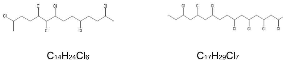
Figure 1: Structures of two representative constituents of CPs with C 14 and C 17 chain lengths
