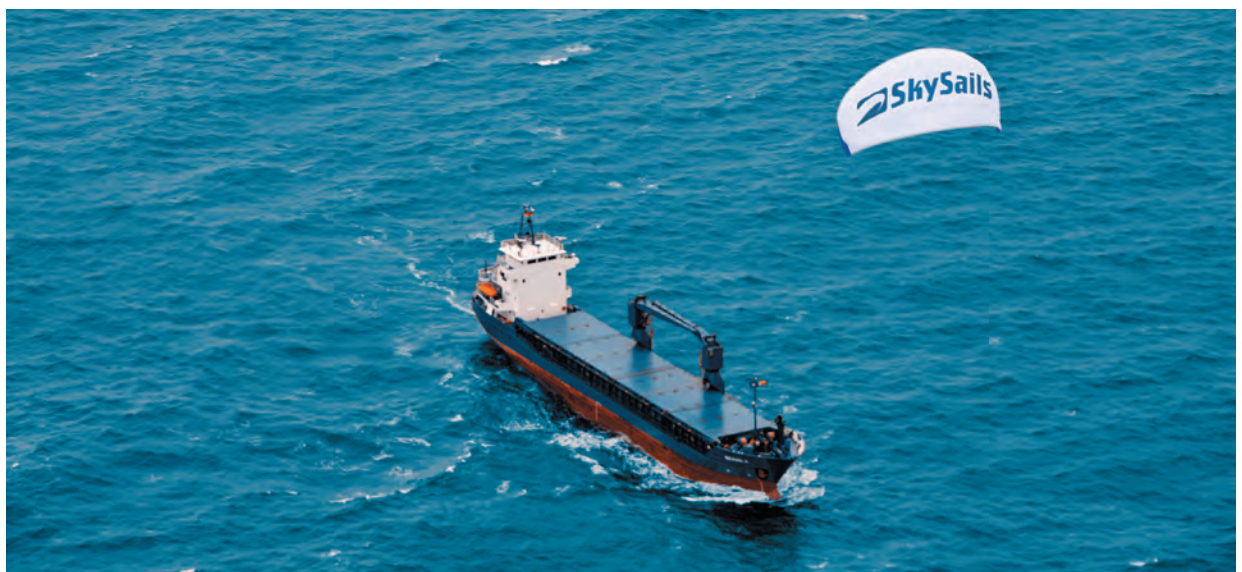
Figure 5.27: Kite providing vessel propulsion assistance. Image courtesy of SkySails Group GmbH [66].
