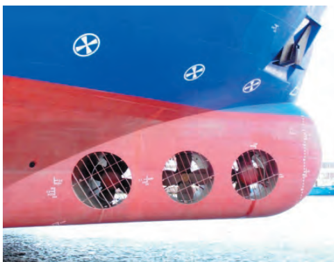
Figure 5.6: Maneuvering thrusters by Dr. Hochhaus/CC BY 3.0.
