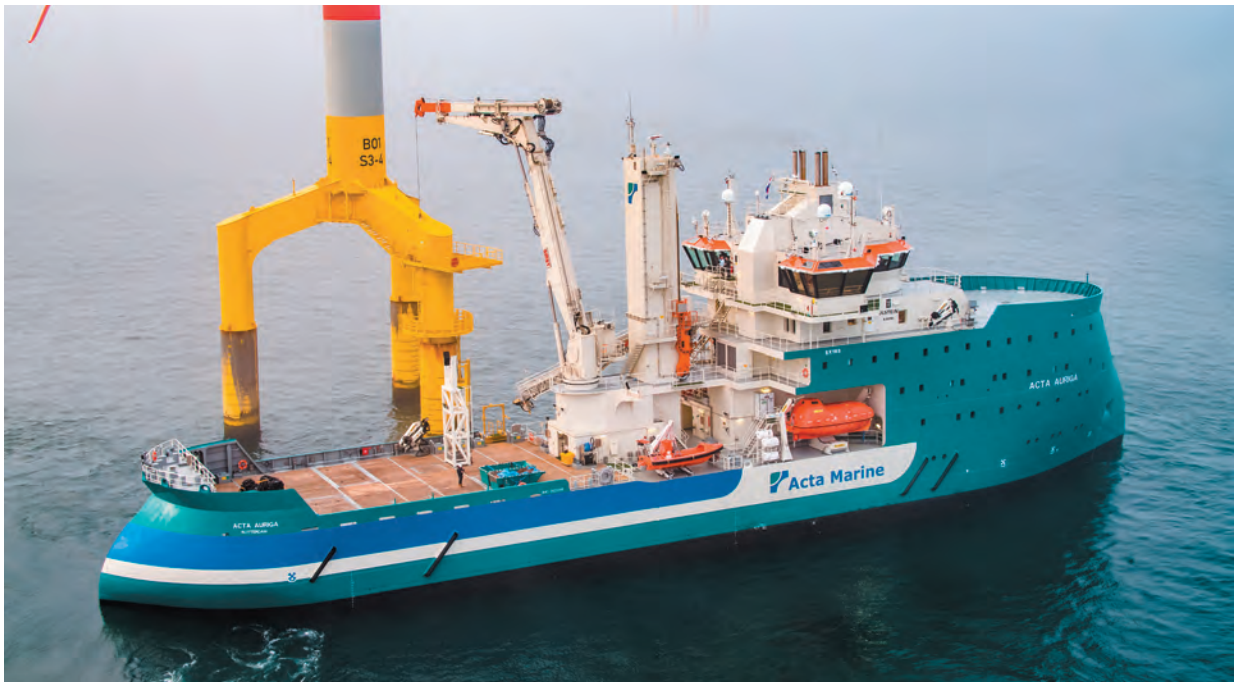
Figure 5.4: The Installation Support Vessel 'Acta Auriga', an Ulstein design including both the X-BOW® and the X-STERN®. Image Courtesy of Acta Marine/Coen de Jong [13].
