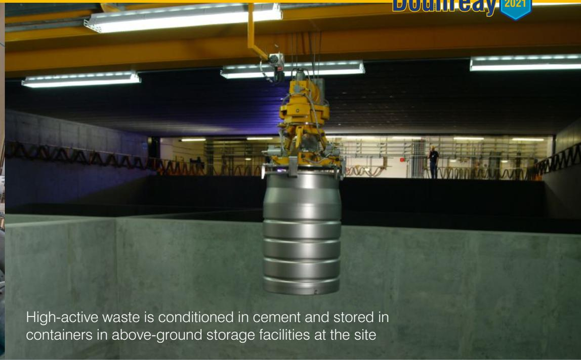
High-active waste is conditioned in cement and stored in containers in above-ground storage facilities at the site
