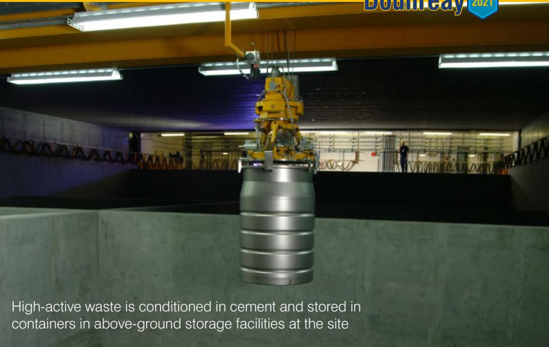
High-active waste is conditioned in cement and stored in containers in above-ground storage facilities at the site
