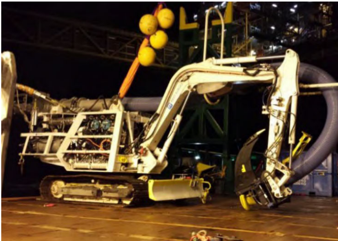
Figure 3-7 Seabed Excavator on Deck (Scanmachine)
