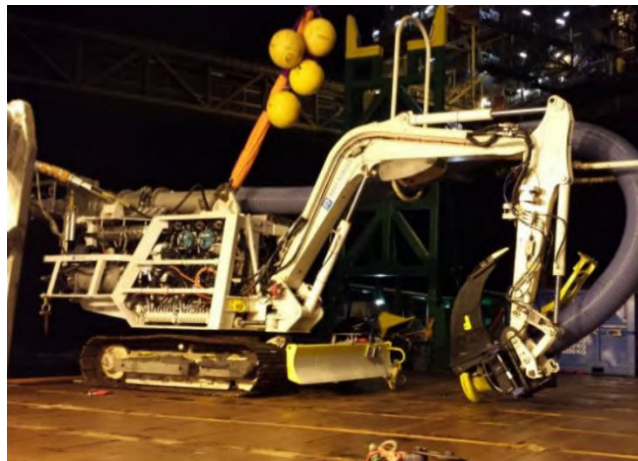
Figure B.11 – Subsea Excavator on Deck (Scanmachine)
