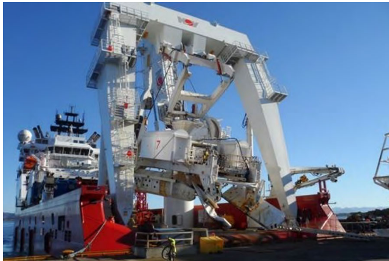
Figure B.19 – Backfill plough
