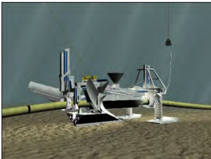
Figure B.17 – Loading pipeline into VMP
