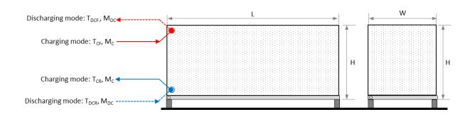
We anticipate the thermal storage to be available in 10, 20 and 40ft shipping container modules. These units will follow a similar configuration and will have the ability to be used in multiples. This will allow the storage to be easily retrofitted into growing plants.
