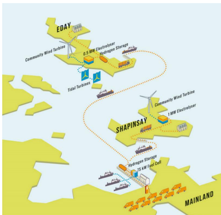
Figure 1. The Orkney hydrogen ecosystem showing production of hydrogen on the island of Eday, and its transport via ferry to the Orkney mainland. (Image from (BIG HIT, 2018)).
