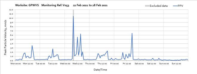
Note: High vibration levels measured at 08:00 on Wednesday 24<sup>th</sup> February 2021 was due works undertaken close to the monitor and are not representative of HS2 construction vibration.
