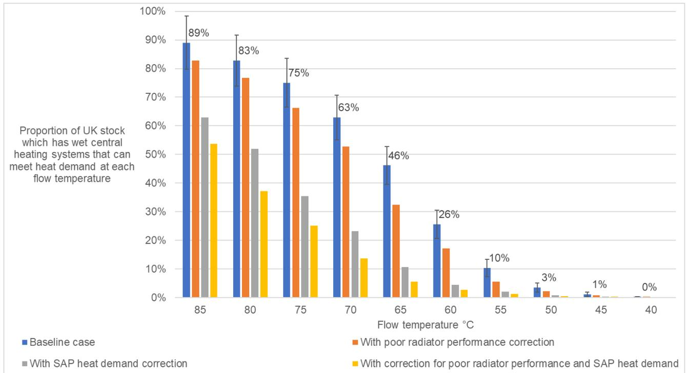
**Figure 2- Proportion of UK dwellings, with wet central heating systems, that could meet peak heat demand (kW) at each flow temperature. (Average temperature across sample for the peak is -3.5°C. Error bars give 95% statistical confidence interval).**
