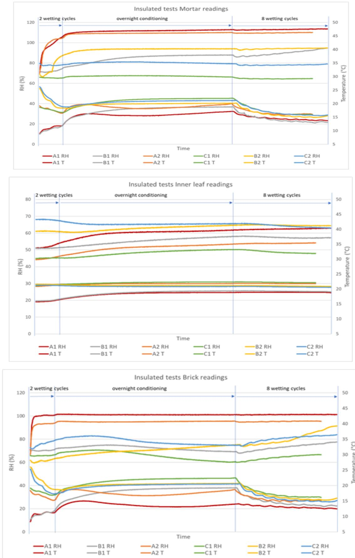
Figure 8: RH and temperature variation in outer wall mortar and brick, and inner leaf brick in **insulated** walls
