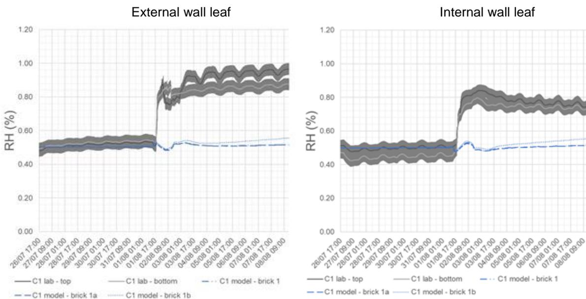
Figure 15: Model predictions (dashed lines) versus laboratory measurements (solid lines, with  $\pm 3.5\%$  declared RH measurement error) of RH behind the external wall leaf (left), and internal wall leaf (right), assuming treated bricks in an uninsulated wall
