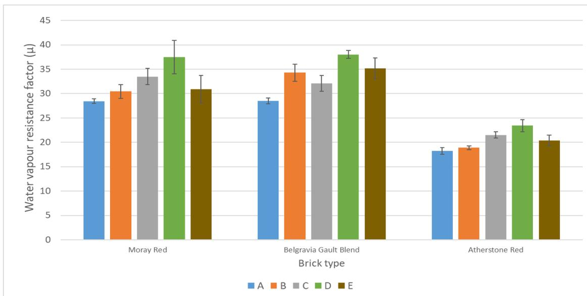
Figure 4: Water vapour resistance factor ( $\mu$ ) of masonry specimens with different brick types and various waterproofing treatments
