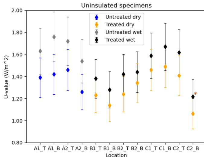
Figure 10: U-values for uninsulated untreated (walls A) and treated (walls B and C) wall samples
