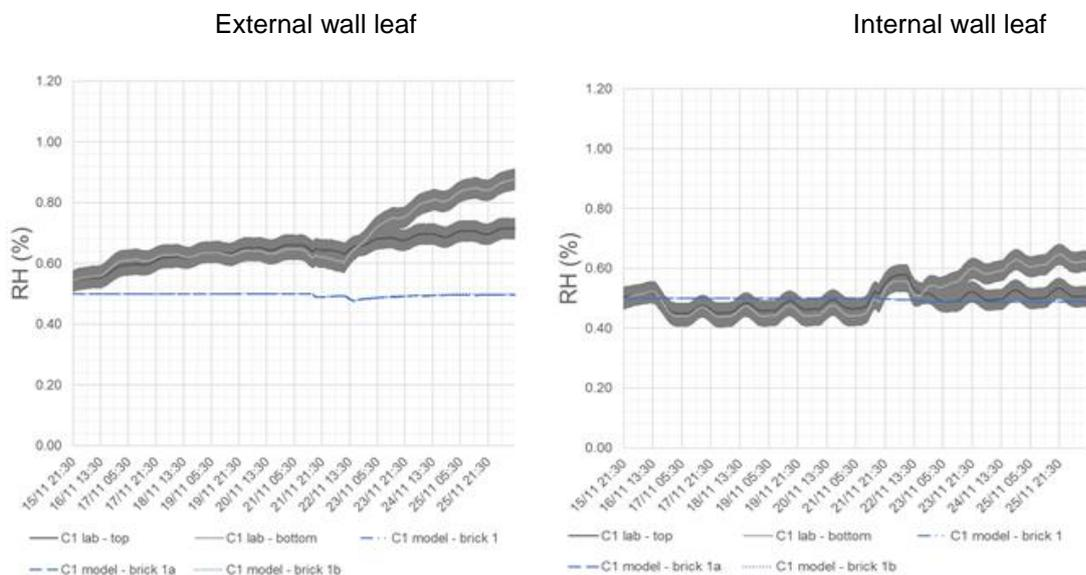
Figure 17: Model predictions (dashed lines) versus laboratory measurements (solid lines, with  $\pm 3.5\%$  declared RH measurement error) of RH behind the external wall leaf (left), and internal wall leaf (right), assuming untreated bricks in an insulated wall
