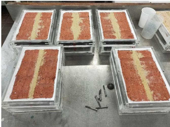
Figure 3: Water vapour permeability test set up, with the mortar and brick samples placed over wet cups
