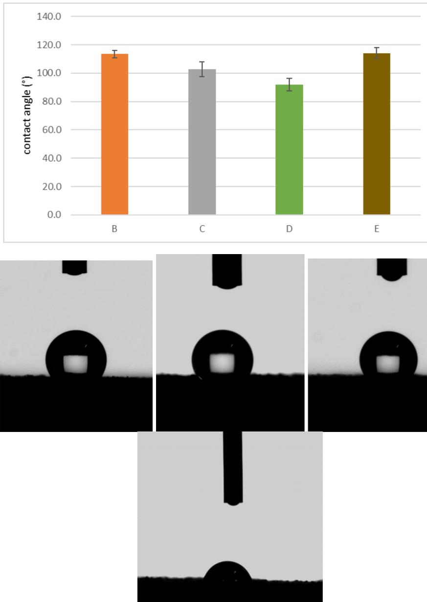
Figure 5: Average water contact angles for each treated specimen and water drop on specimens treated with a) product B b) product C, c) product D, d) product E
