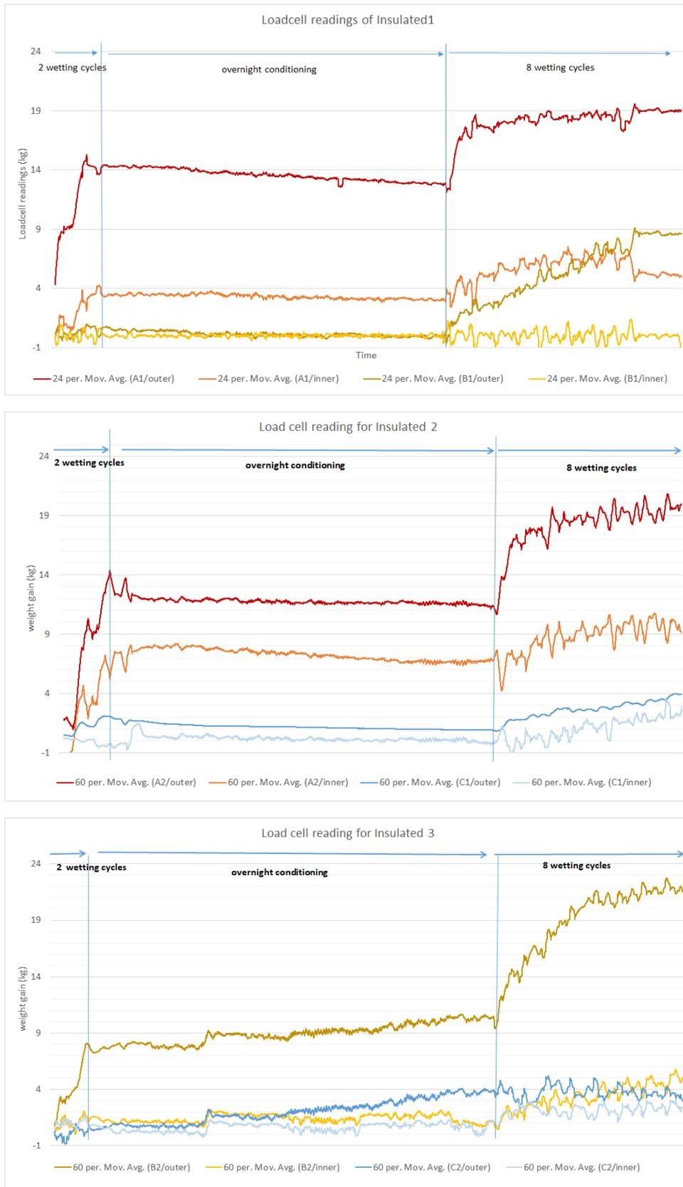
Figure 9: Load cell weight gain of outer and inner wall leaves in **insulated** walls
