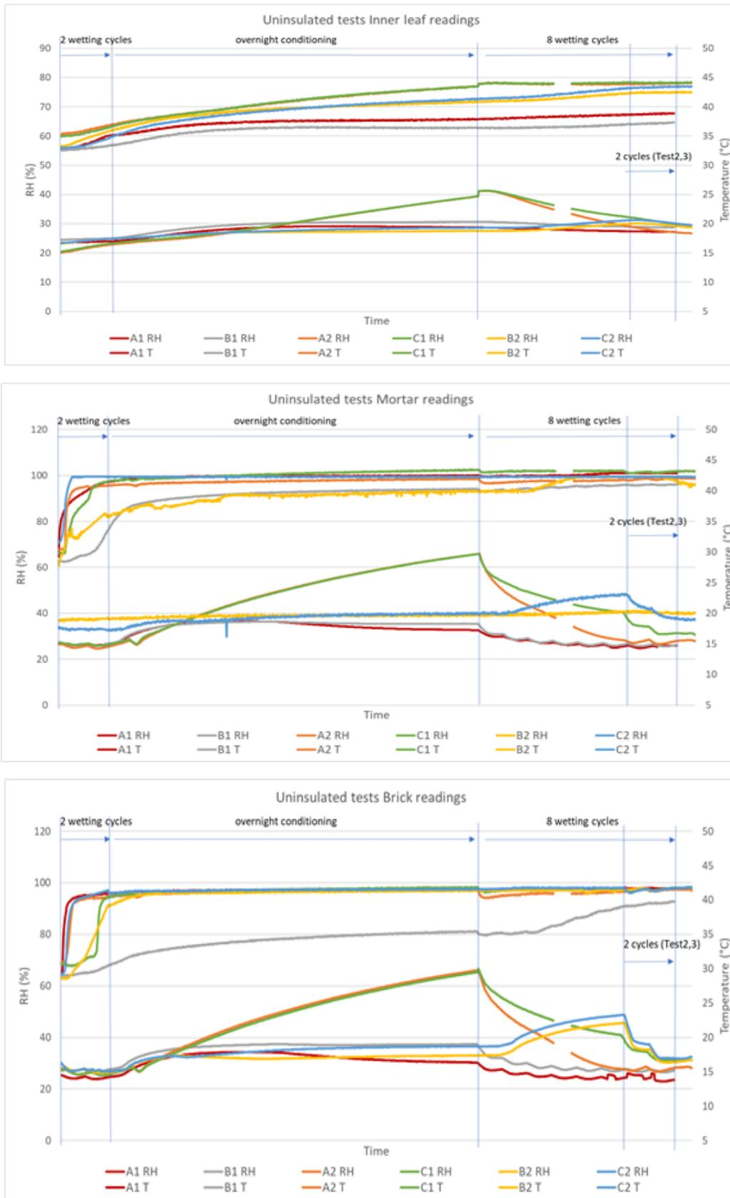
Figure 7: RH and temperature variation in outer leaf mortar and brick, and inner leaf brick in **uninsulated** walls
