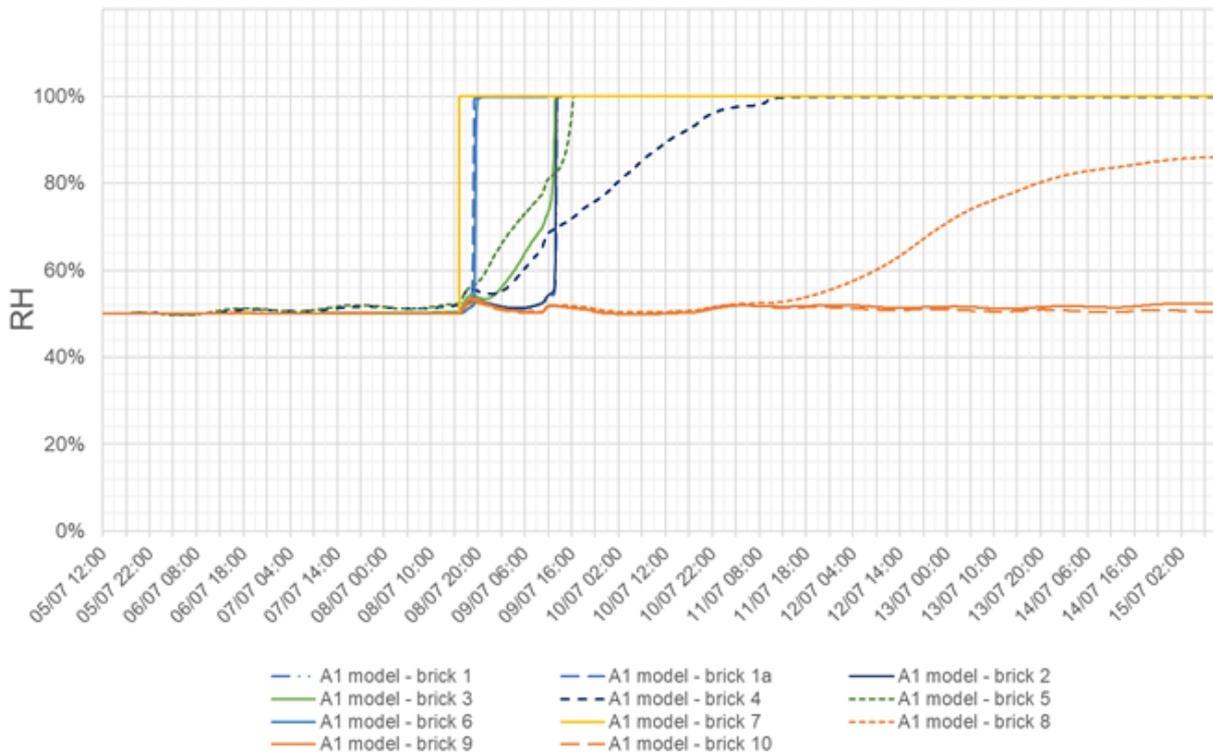
Figure 13: Simulated RH behind an external wall leaf, assuming untreated bricks from the Delphin software
