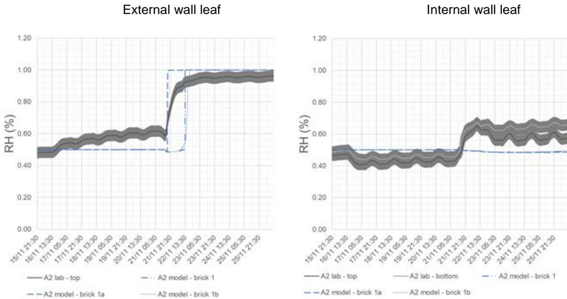
Figure 16: Model predictions (dashed lines) versus laboratory measurements (solid lines, with  $\pm 3.5\%$  declared RH measurement error) of RH behind the external wall leaf (left), and internal wall leaf (right), assuming untreated bricks in an insulated wall
