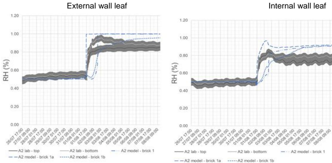
Figure 14: Model predictions (dashed lines) versus laboratory measurements (solid lines, with  $\pm 3.5\%$  declared RH measurement error) of RH behind the external wall leaf (left), and internal wall leaf (right), assuming untreated bricks in an uninsulated wall
