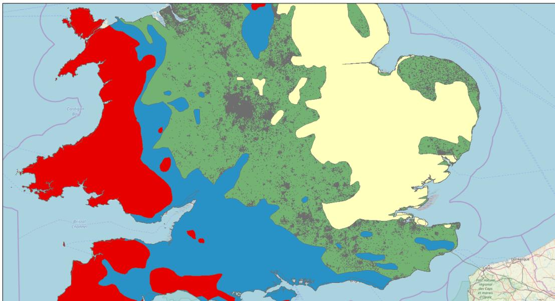
Figure 19: Buildings in England (grey, from Geofabrik database) located in exposure zone 2 (green zone)
