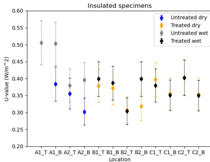
Figure 11: U-values for insulated untreated (walls A) and treated (walls B and C) wall samples
