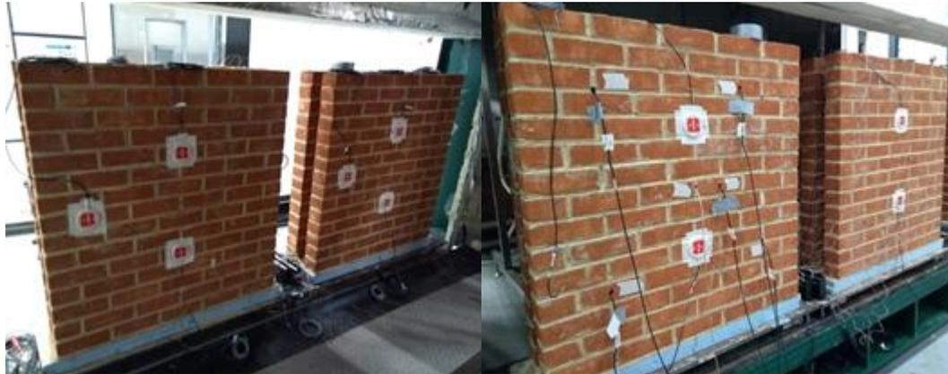
Figure 2: Cavity wall specimen instrumentation for the external (left) and internal (right) simulated environments
