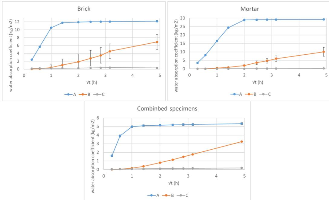
Figure 6: Weight change of various samples in absorption test
