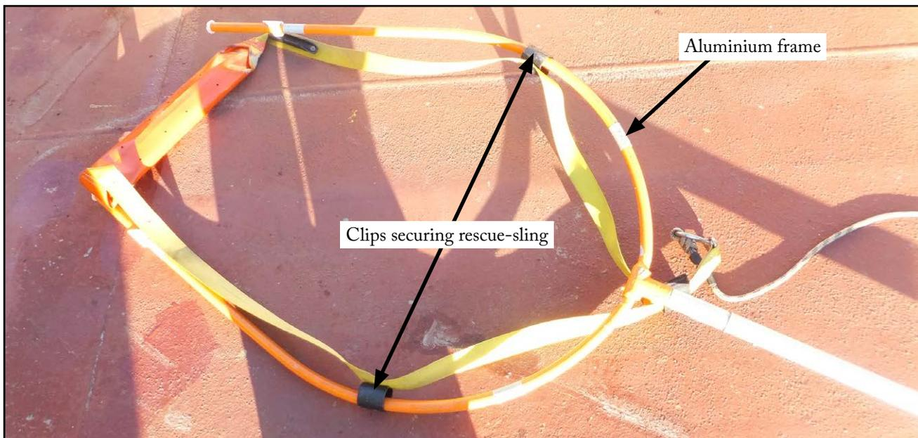
Figure 2: Man overboard rescue device with detachable strop
