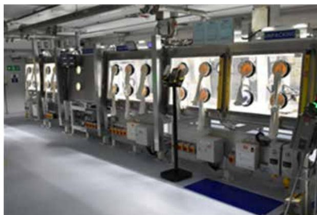
Modified glovebox line for uranium processing
