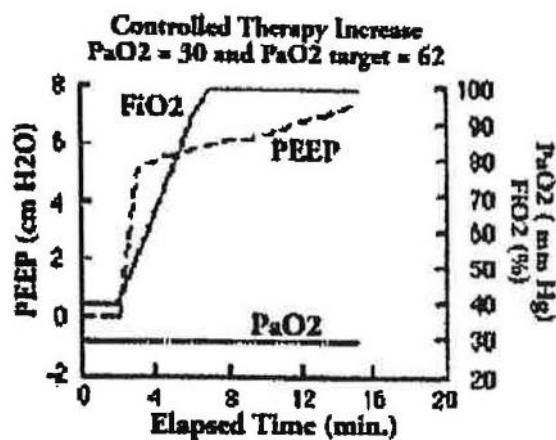
Figure 6. Controller's open loop response to "Threatening" patient PaO<sub>2</sub>.
