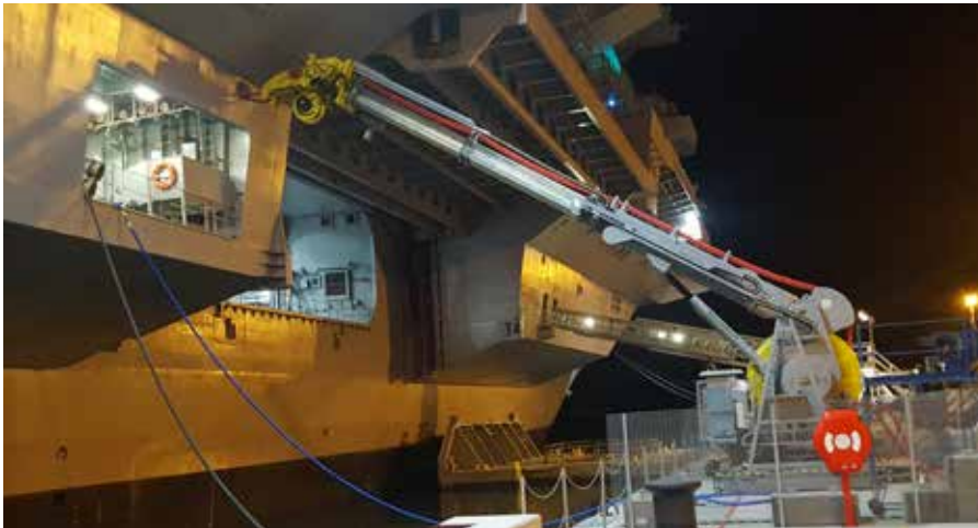
A telescopic cable boom connection powers the carriers when berthed © Andy Amor
