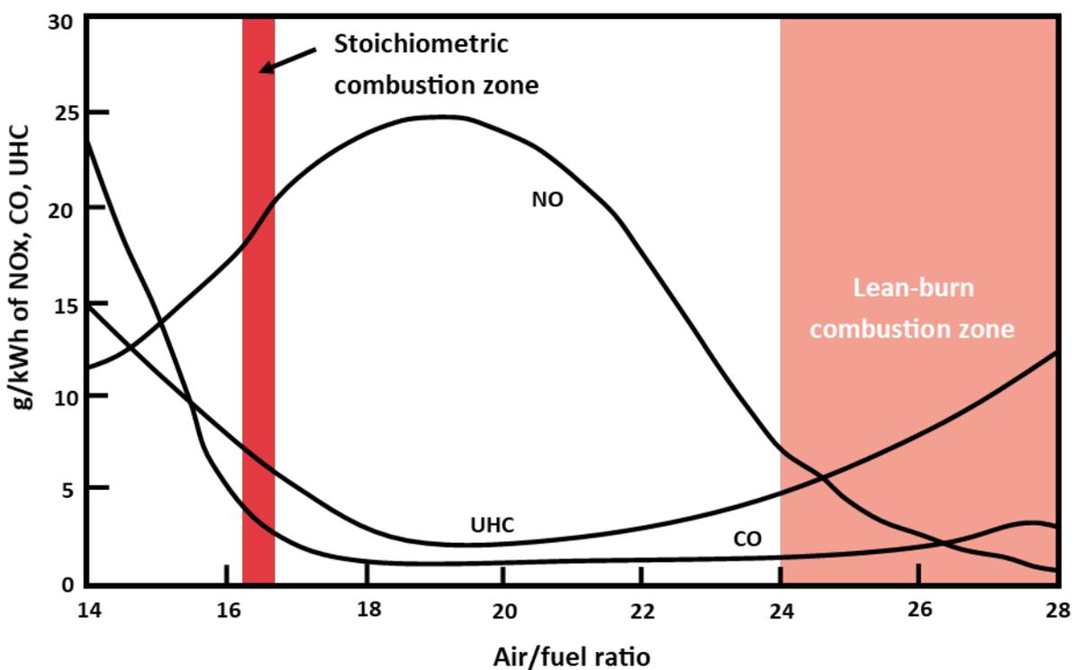
**Figure 16 - Emissions at Differing Air-to-Fuel Ratios**
