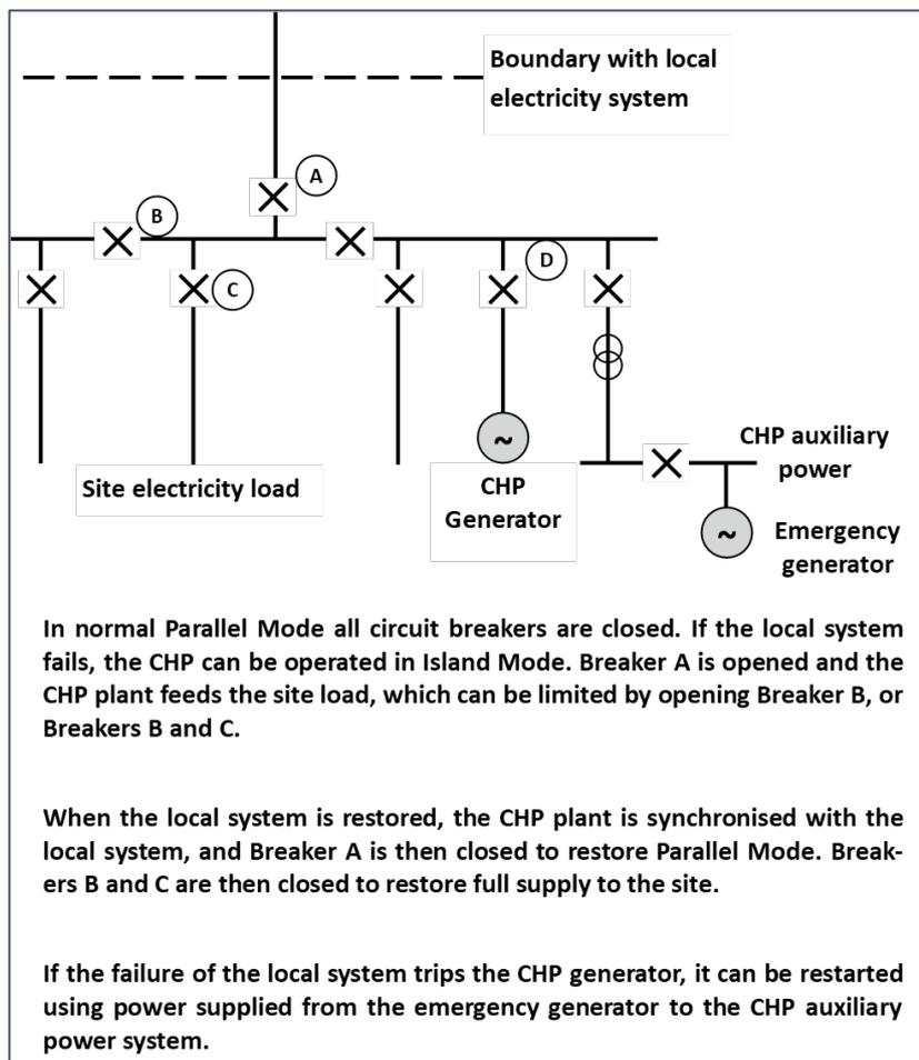
Figure 14 - Circuit Breaker Schematic
