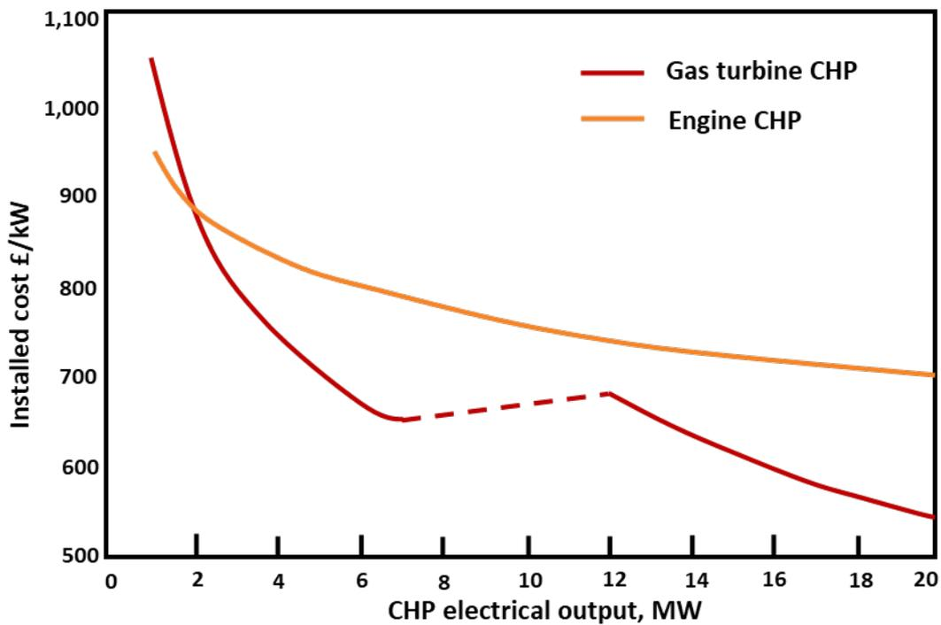
**Figure 1: Installed cost of CHP with increasing electrical capacity**
