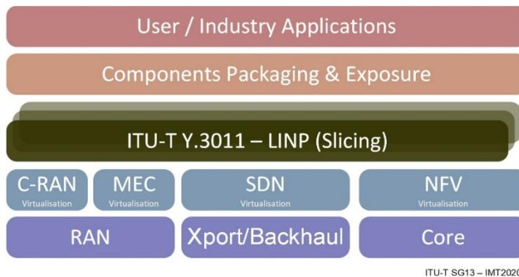
Further layers of abstraction are built on top of the Virtualisation Layer and are the means by which network services are instantiated as collections of software components; representing virtualised network functions, which are then orchestrated to either compose or support user applications.
