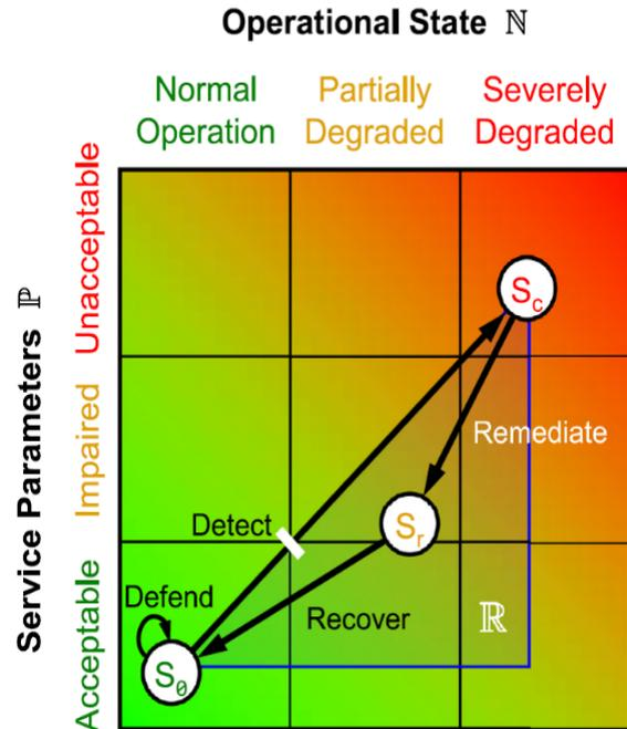
The  $D^2R^2$  ResiliNets strategy (Defend, Detect, Remediate and Recover) is overlaid on the figure. The initial state of acceptable service under normal operations is  $S_\theta$ . As long as resilience defences hold this will remain the case.
