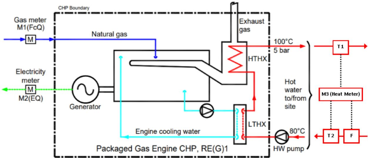
NOTE: Heat meter M3 is not needed when the RE is <500kWe capacity. Heat output can be determined by multiplying the power output (from M2) by the design heat to power ratio of the engine. Similarly, if the RE is <500kWe, the fuel can be determined by multiplying the power output (from M2) by the design power efficiency the engine (if the engine is on the CHPQA Unit List).
