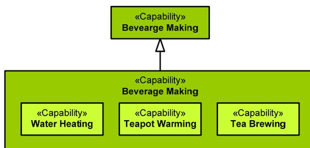
The ability to model capabilities as being components of other capabilities is part of the more general MODAF approach to modelling *dependencies* between capabilities.
