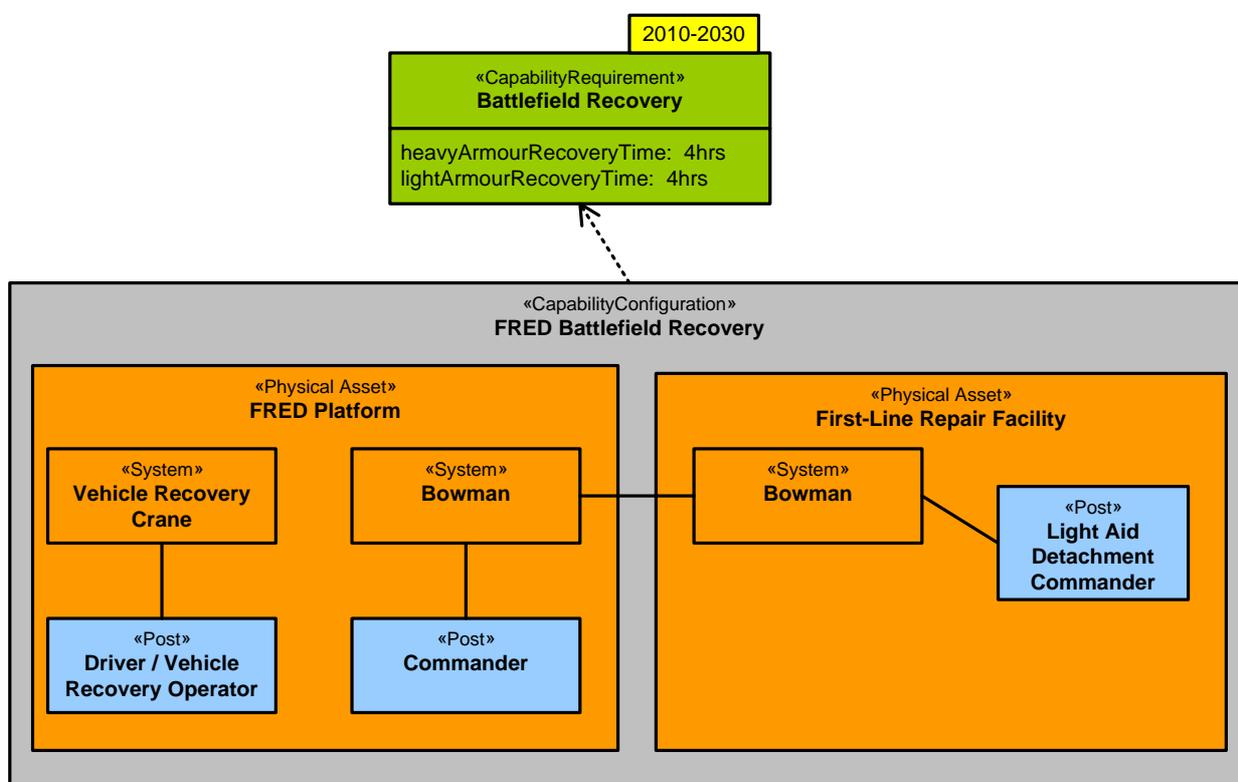
The final aspect of capability that is covered by MODAF is the concept of actual, physical capability, ie a real world instance of a capability configuration.
