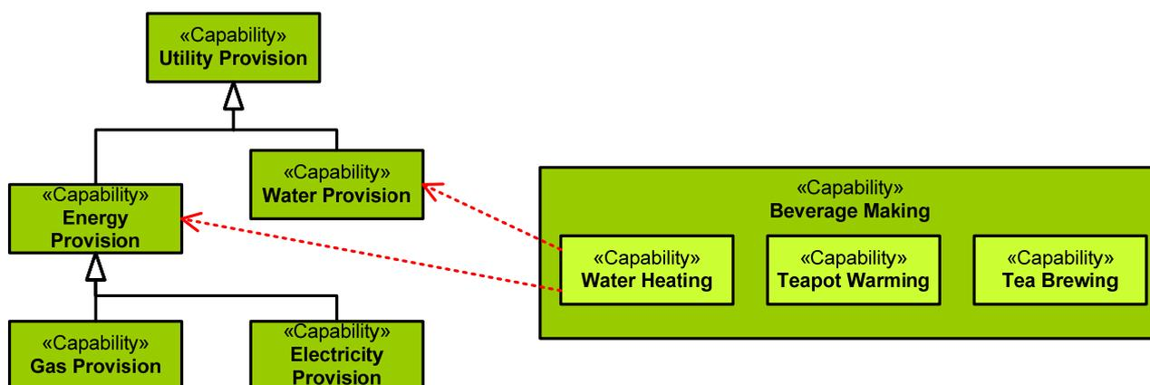
The dotted arrow points to the capability upon which another capability depends; ie the dotted line should read from tail to head: “depends on”.
