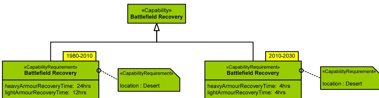
The capability requirements specify performance metrics – in this case, the required recovery time is greatly reduced. Once a taxonomy of capabilities and capabilities requirements have been defined, these can be re-used across a number of architectures. Operational architectures can apply capabilities to scenarios and plans:
