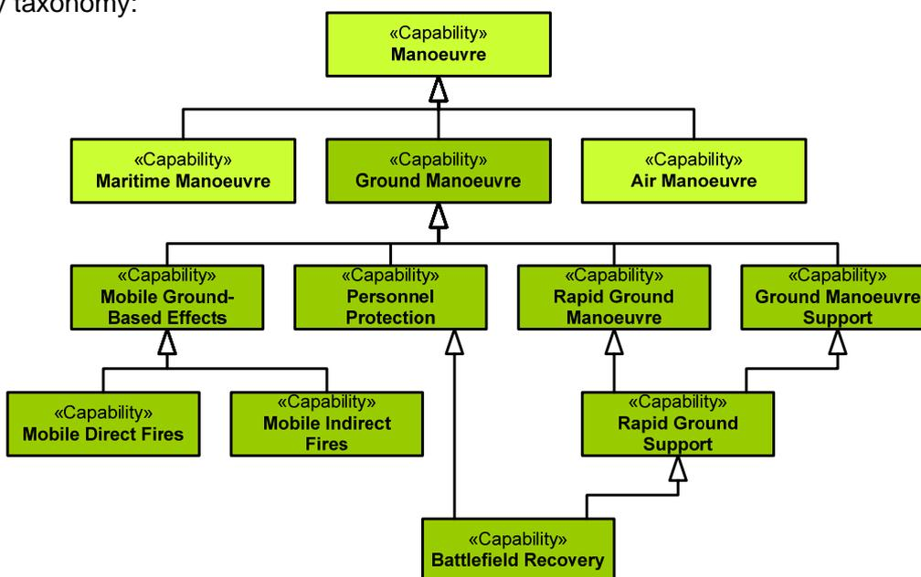
The diagram above (which uses a UML notation) shows a specialisation hierarchy of capabilities. Note that some capabilities specialise from more than one parent, for example, **Rapid Ground Support** is both a **Rapid Ground Manoeuvre** and a **Ground Manoeuvre Support** capability.
