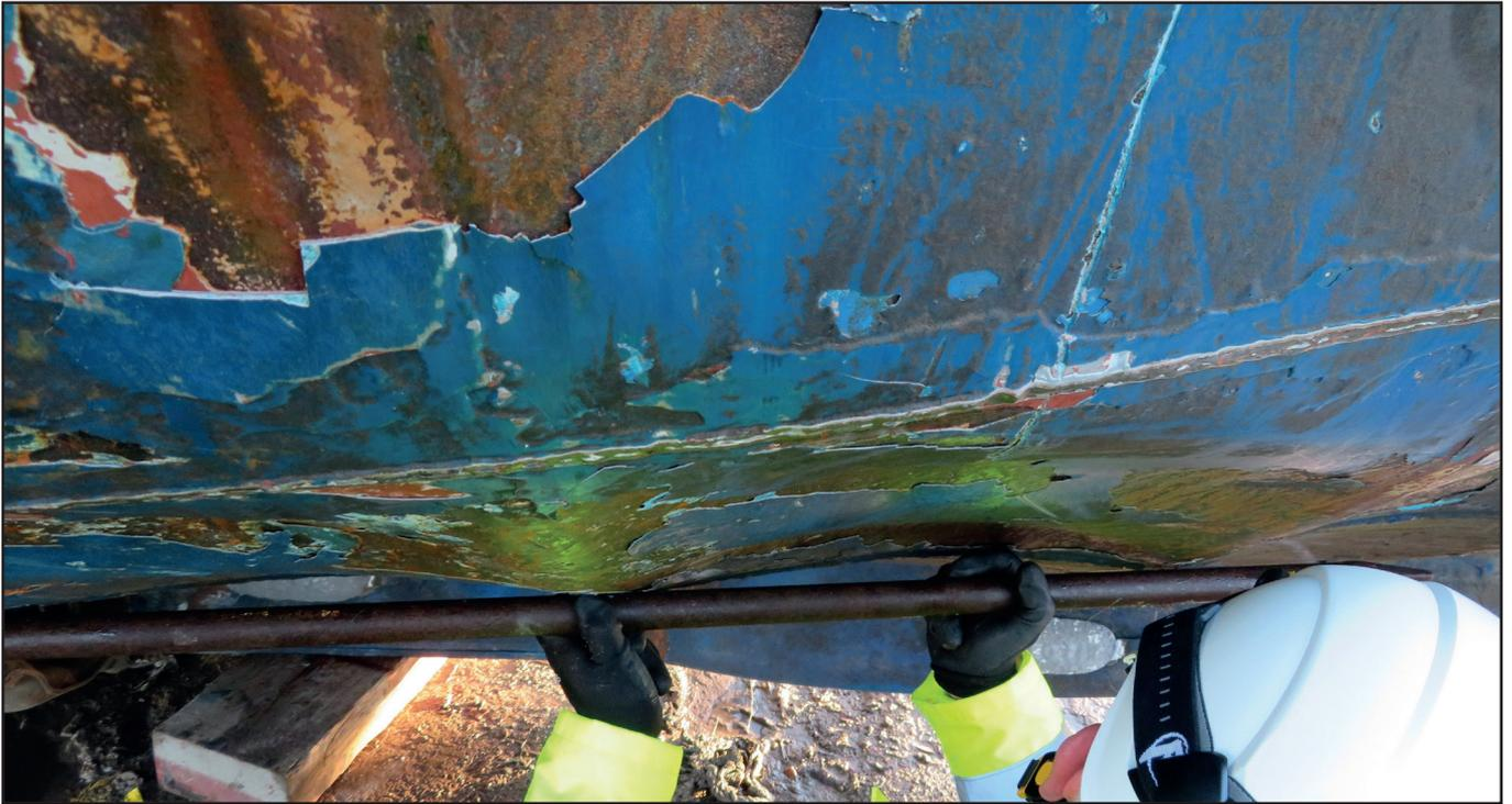
**Figure 3:** Detail of shell plating damage showing coating loss and indentation between internal frames
