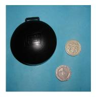
Figure 2: A DRPS ADS radon detector
