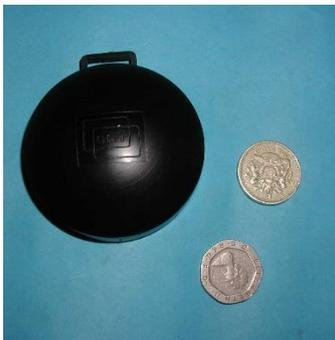
*Figure 2: A DRPS ADS radon detector*
