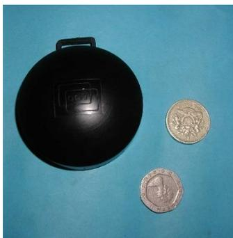
*Figure 2: A DRPS ADS radon detector*
