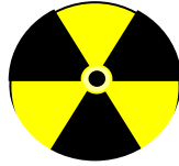
Figure 2 Standard radiation trefoil. Colour of symbol: black on yellow or white background.
