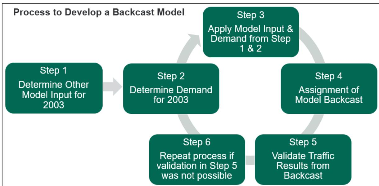
**Figure 50 Process to Develop a Backcast Model**
