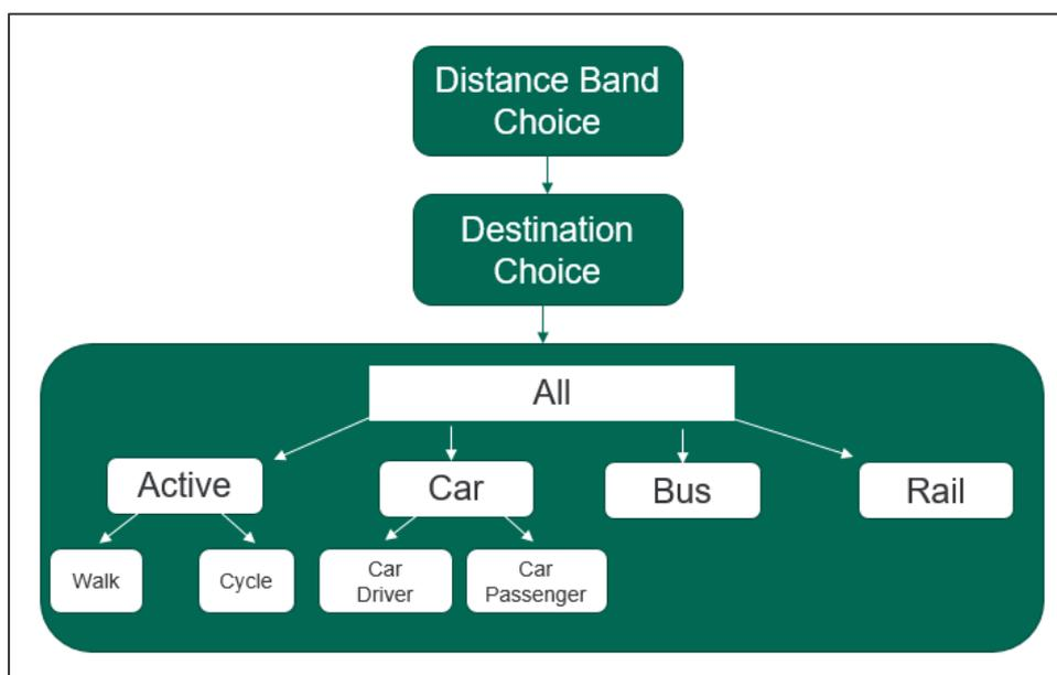
**Figure 6: Diagram of the NTM choice model**
