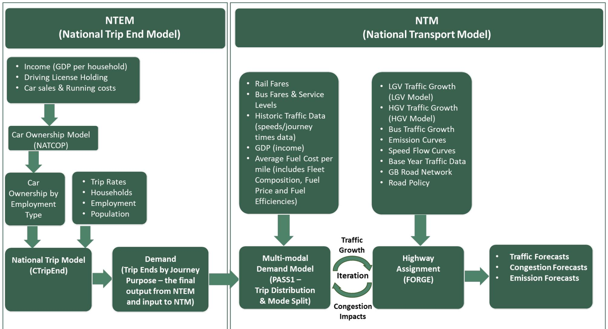
Figure 2: Inputs and Connectivity of the National Trip End Model and National Transport Model
