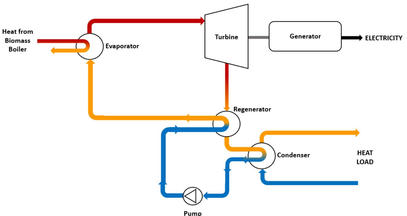
ORCs are designed to operate at lower temperatures than conventional steam cycles. Feed fluids vary between 80°C and 120°C and return temperatures are within 50°C and 100°C. Temperature differentials can vary between 15°C and 50°C dependant on the design. The higher the temperature differential, the higher the system efficiency.
