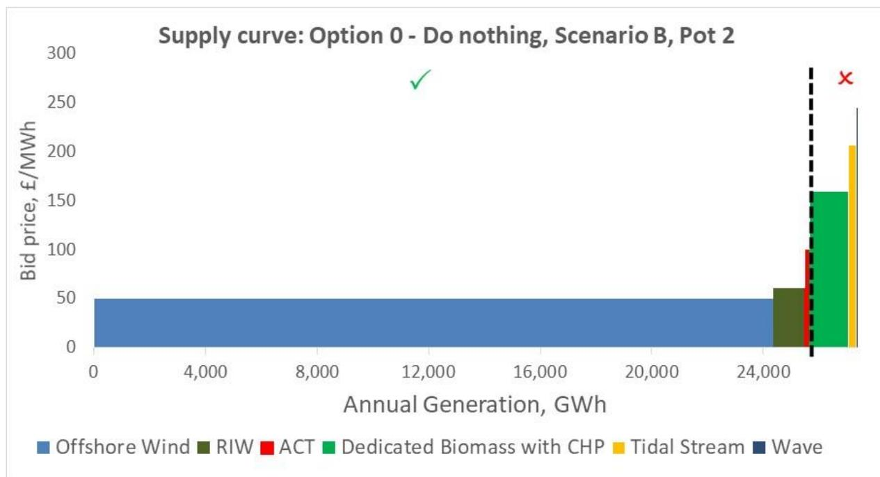
Figure 1 illustrates Scenario B, Pot 2, under Option 0: do nothing. In this scenario offshore wind, RIW and ACT projects are successful. Floating offshore wind is not classified as a separate technology and so does not appear in the bidding pipeline. All other Pot 2 technologies are assumed to be uncompetitive.
