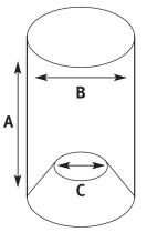
A: The trap must be no longer than 600mm
