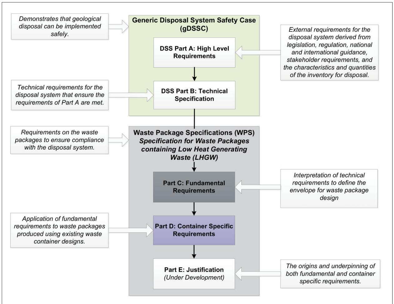
To support safe delivery of a fully operational GDF, RWM has developed the generic Disposal System Safety Case (gDSSC), which details the conceptual designs for a GDF and how this will ensure the safe disposal of radioactive waste. The gDSSC is comprised of 33 documents, including the Disposal System Specification Part A and Part B, which can be found at [rwm.nda.gov.uk/publications](http://rwm.nda.gov.uk/publications). An overview of all documents within this suite is provided in DSSC/101/01.
