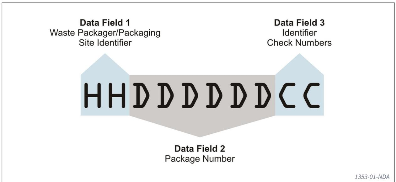
Figure 12: Permissible OCR-A characters that are to be used in the production of a waste package identifier.
