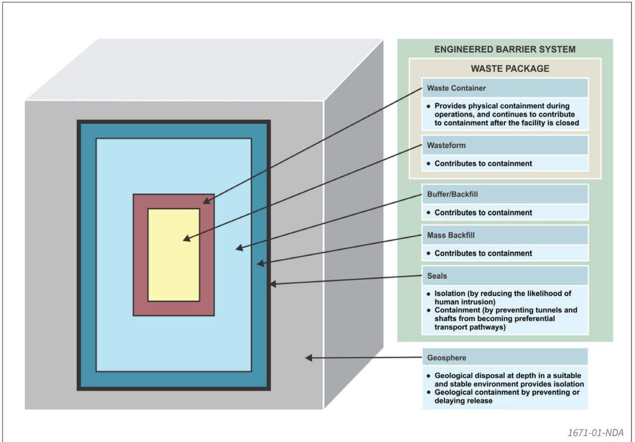
Figure 6: Schematic representation of a waste package in which an immobilisation material has been used. Together, the wasteform (consisting of the waste and immobilisation material) and the waste container, provide the primary layers of containment in the disposal system.
