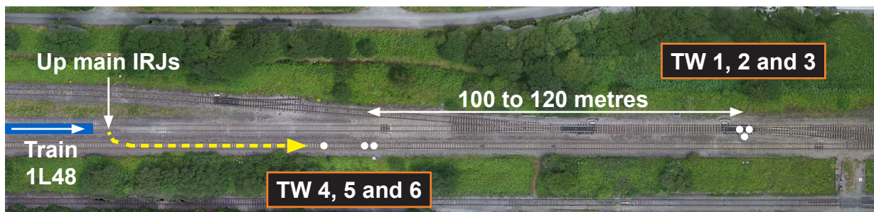
Figure 4: Position of workers immediately before the accident
