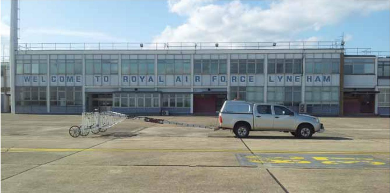
The towed magnetometer array at RAF Lyneham, surveying as part of the transition program © Crown
