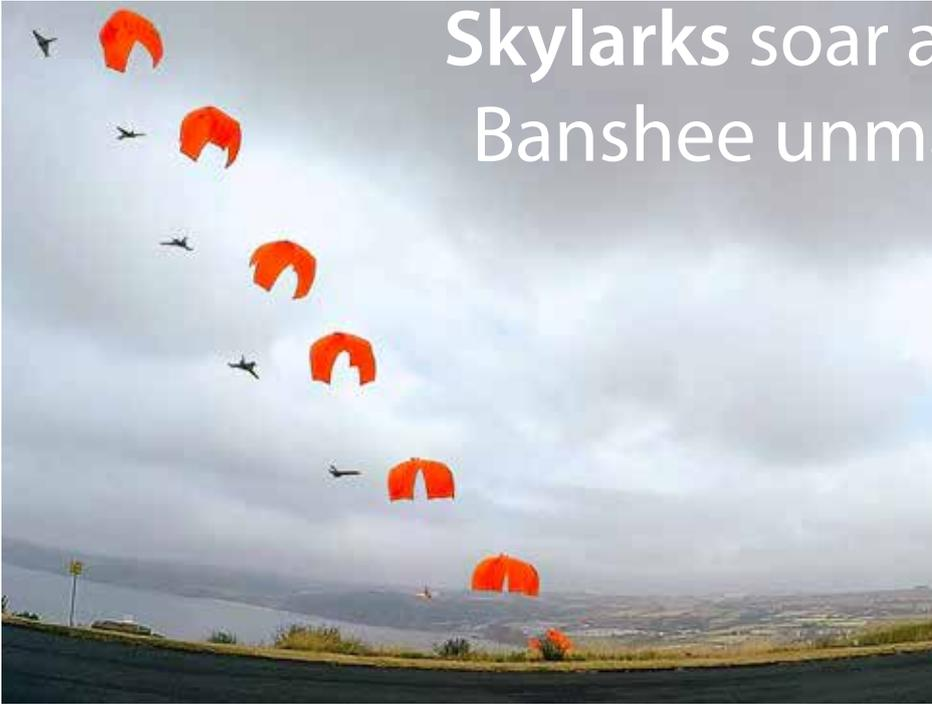
Banshee Whirlwind target parachute recovery phase – a time delayed image © QinetiQ Ltd
