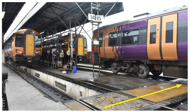
Figure 9: Trains positioned as at the time of the accident during the RAIB reconstruction. The obstructed walking route across number 15 siding is indicated.
