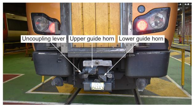
Figure 5: BSI autocoupler fitted to Class 172 unit
