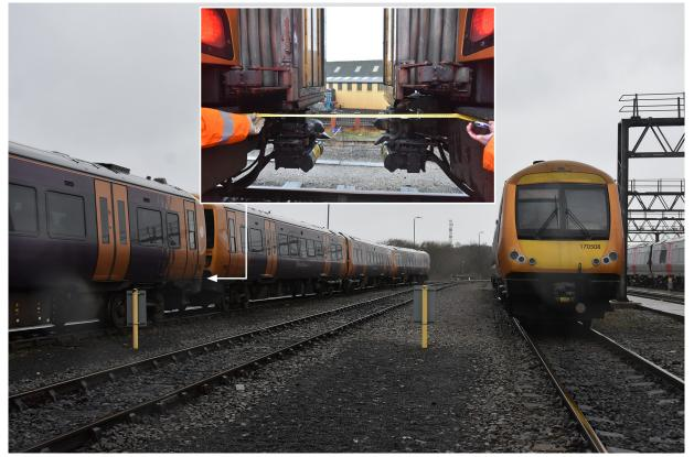
Figure 13: Trains on number 15 siding as positioned during the RAIB reconstruction. Inset shows the gap between the two Class 172 units
