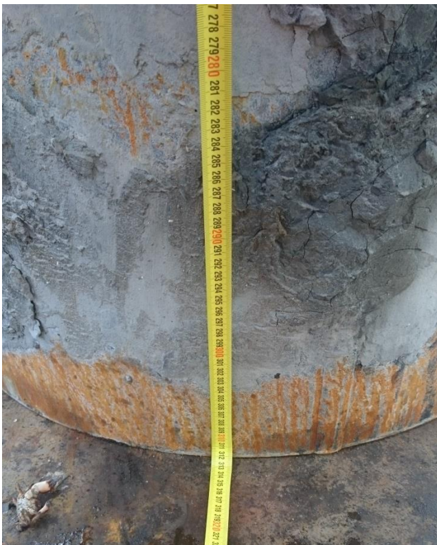
Fig 1.6 – Photos illustrating Stiff grey clay stuck to bottom 1.5 - 2.0m of cut WHPS pile
