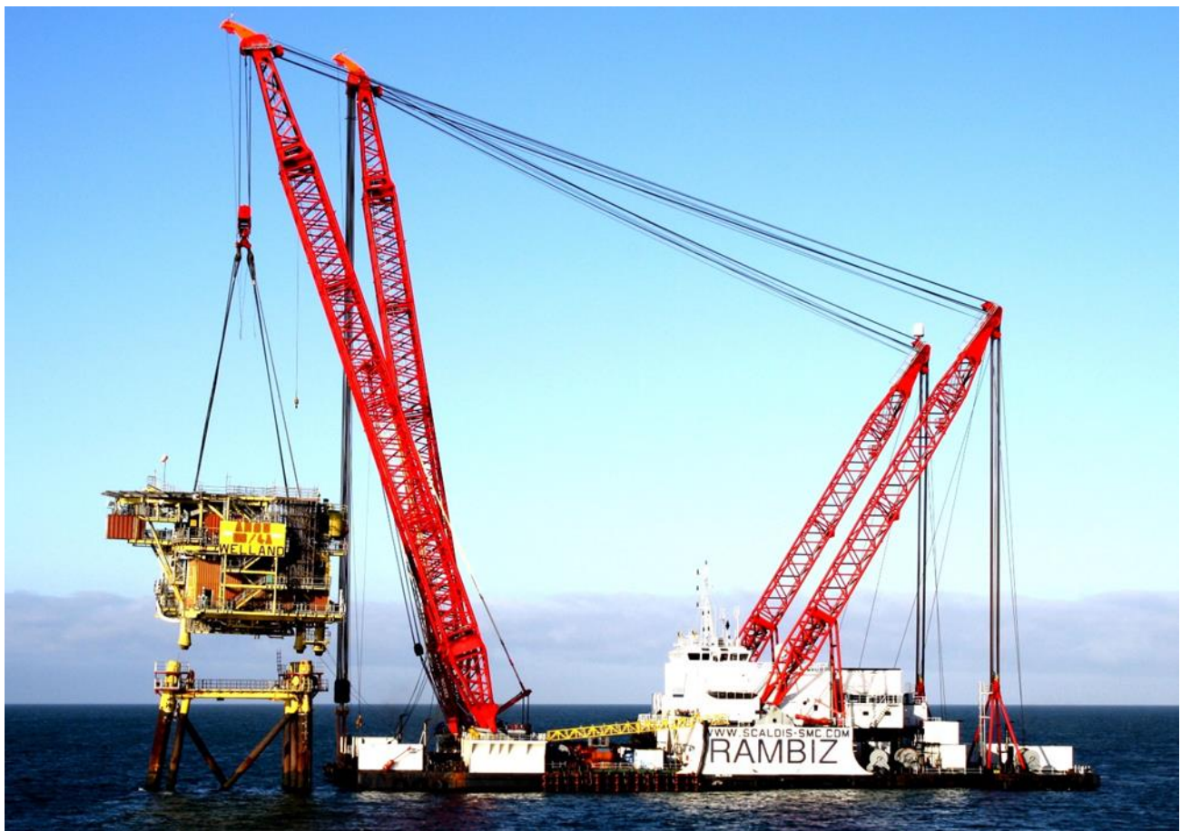
Fig 1.7 - Rambiz HLV Lifting Welland Topside
