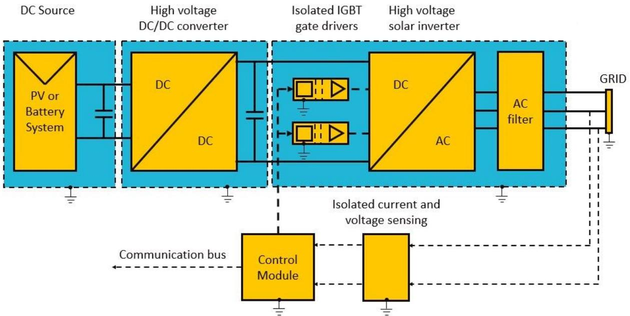
For BESS systems supplied as ‘storage only’, the choice of inverter is the responsibility of the system designer. Installation is more complicated than with a single box integrated BESS solution as the cabling and protection for the DC side between the batteries and the inverter is external to both products. Inverters used for these applications may be offered with 5-10 years warranties.
