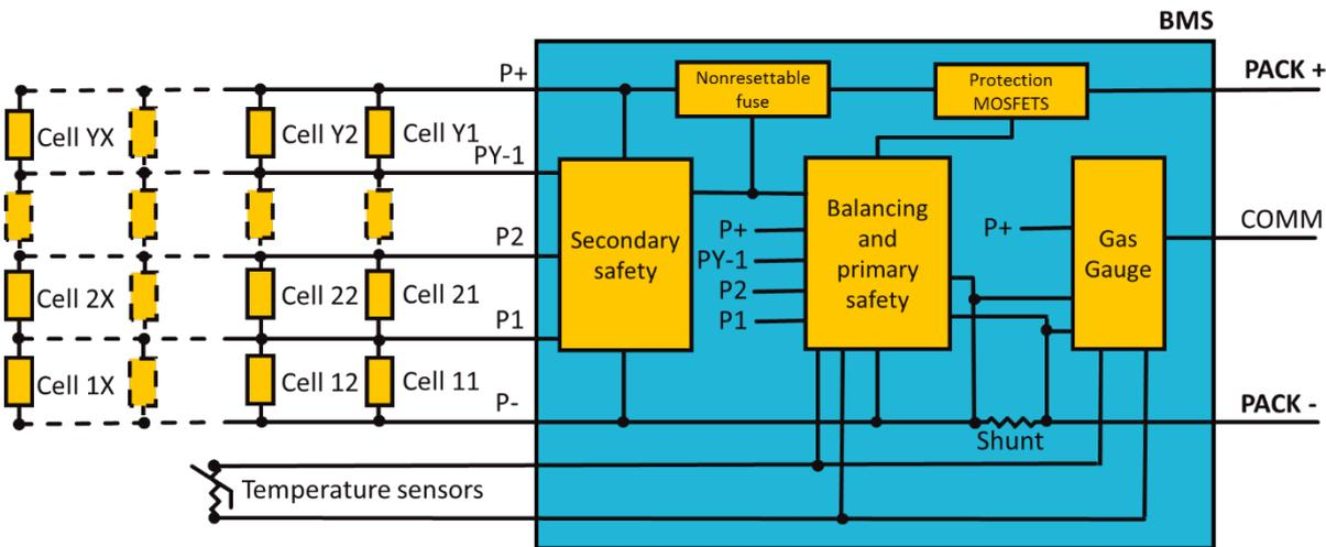
If a BESS is divided into several packs or modules, a BMS similar to the design in Figure 5 is often found in each pack or module. Each BMS communicates alarms and status of each module or pack to a battery management unit or control subsystem (see Figure 1).
