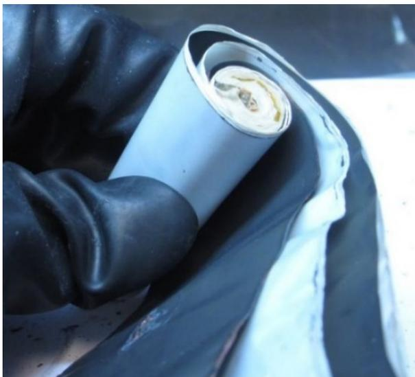
Jelly roll with anode, separator, cathode and separator (left to right) in the picture (© Intertek).
