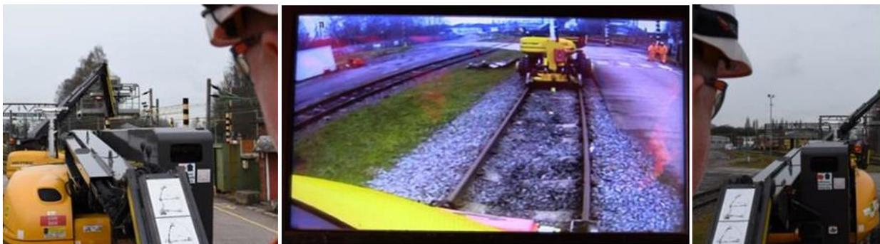
Figure 11: Images taken from MEWP 10, 15 metres from stationary MEWP 3, showing the view from the machine operator's eye level (left), CCTV monitor view (middle) and machine operator eye level view (right) from MEWP 10
