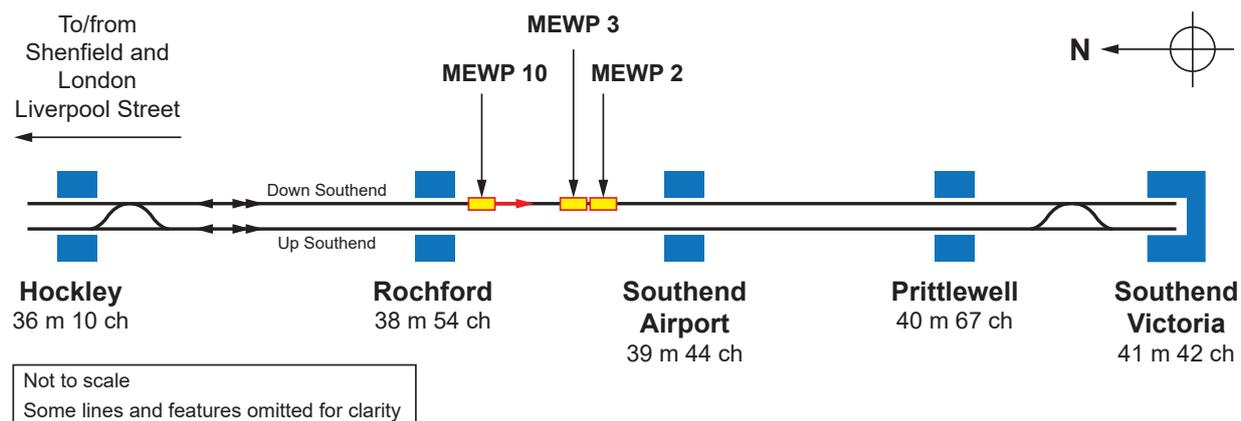
Figure 2: Layout of the track and location of the MEWPs involved in the accident
