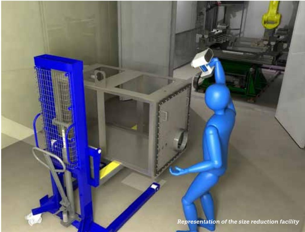
Gloveboxes used for research, development and operations that have come to the end of their life will be decommissioned as part of the site's clean-up programme. Many of these are contaminated with alpha bearing material and current decommissioning plans include manual techniques which are often hazardous and time consuming. There is a driver to address this challenge using alternative technologies to deliver safer, more efficient decommissioning at a lower cost.
