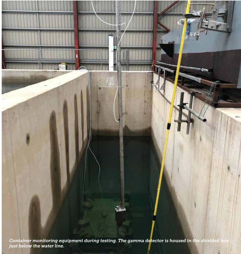
*Container monitoring equipment during testing. The gamma detector is housed in the shielded box just below the water line.*
