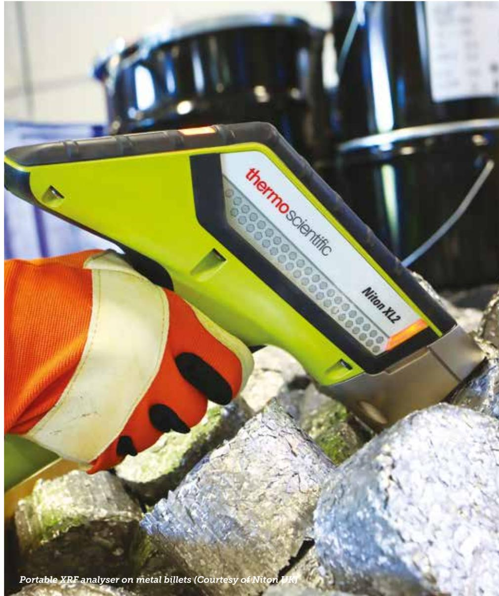
Portable XRF analyser on metal billets (Courtesy of Niton UK)
