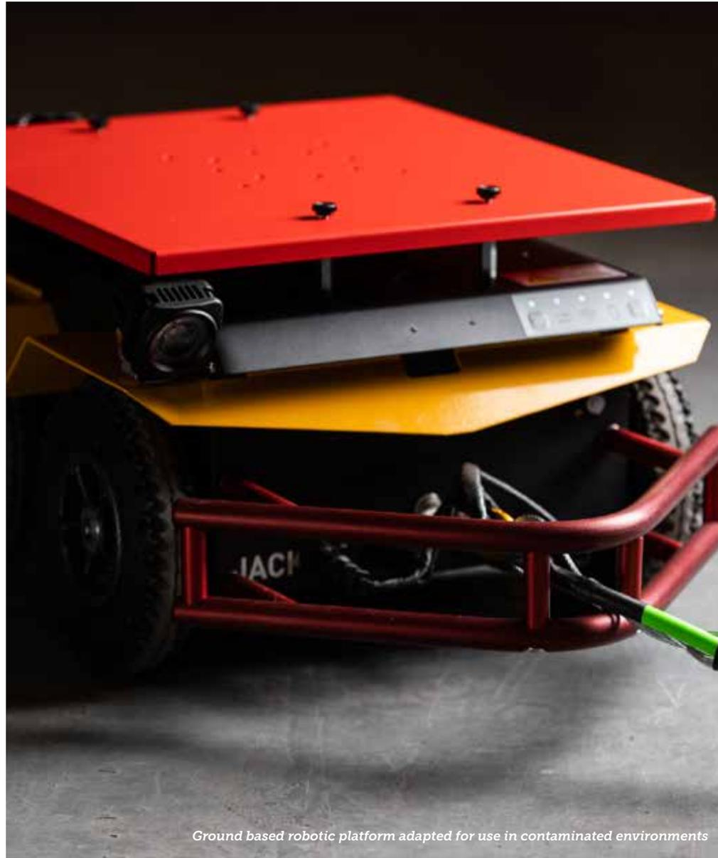
Ground based robotic platform adapted for use in contaminated environments
