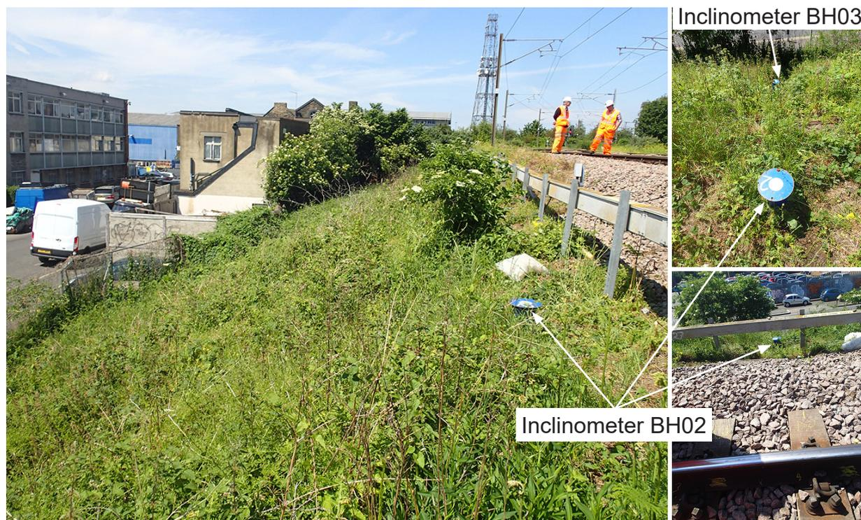
Figure 5: The inclinometer locations on the up-side slope of Mitre Bridge Curve embankment
