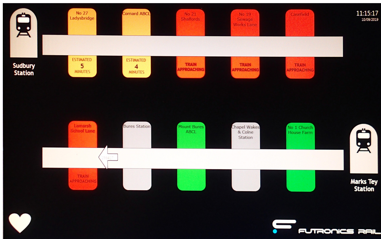
Figure 12: Image of the TAWs interface at Liverpool Street SCC, Witham workstation
