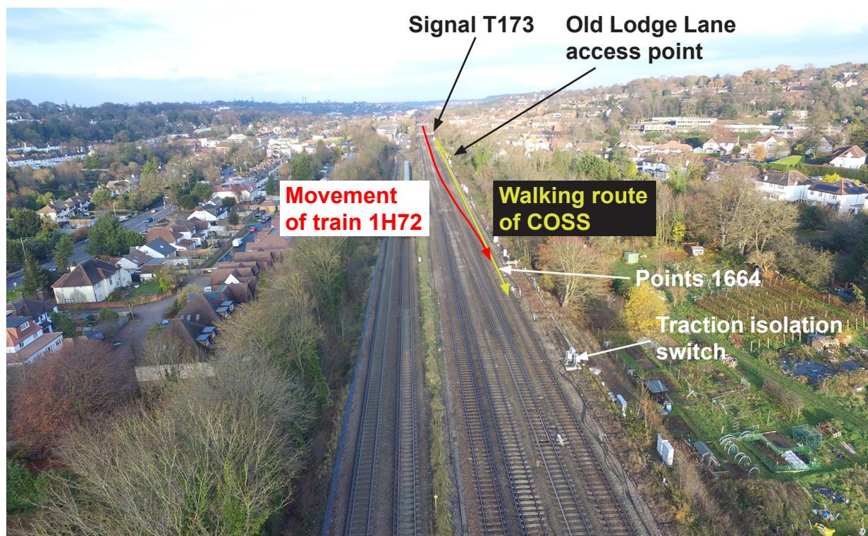
Figure 11: Aerial image showing locations of Old Lodge Lane access point, including the walking route taken by the COSS towards points 1664 (yellow line), the route of train 1H72 (red line) and the location of the trackside equipment
