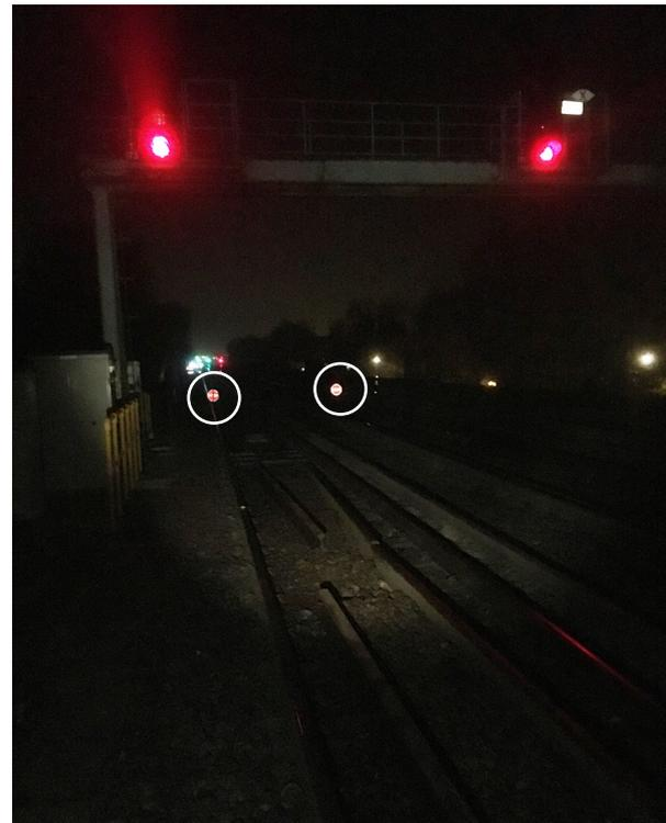
Figure 9: (a) showing a reconstruction of the position of the possession limit boards and detonators and (b) showing signal T173 and the possession limit boards after the accident on 6 November 2018
