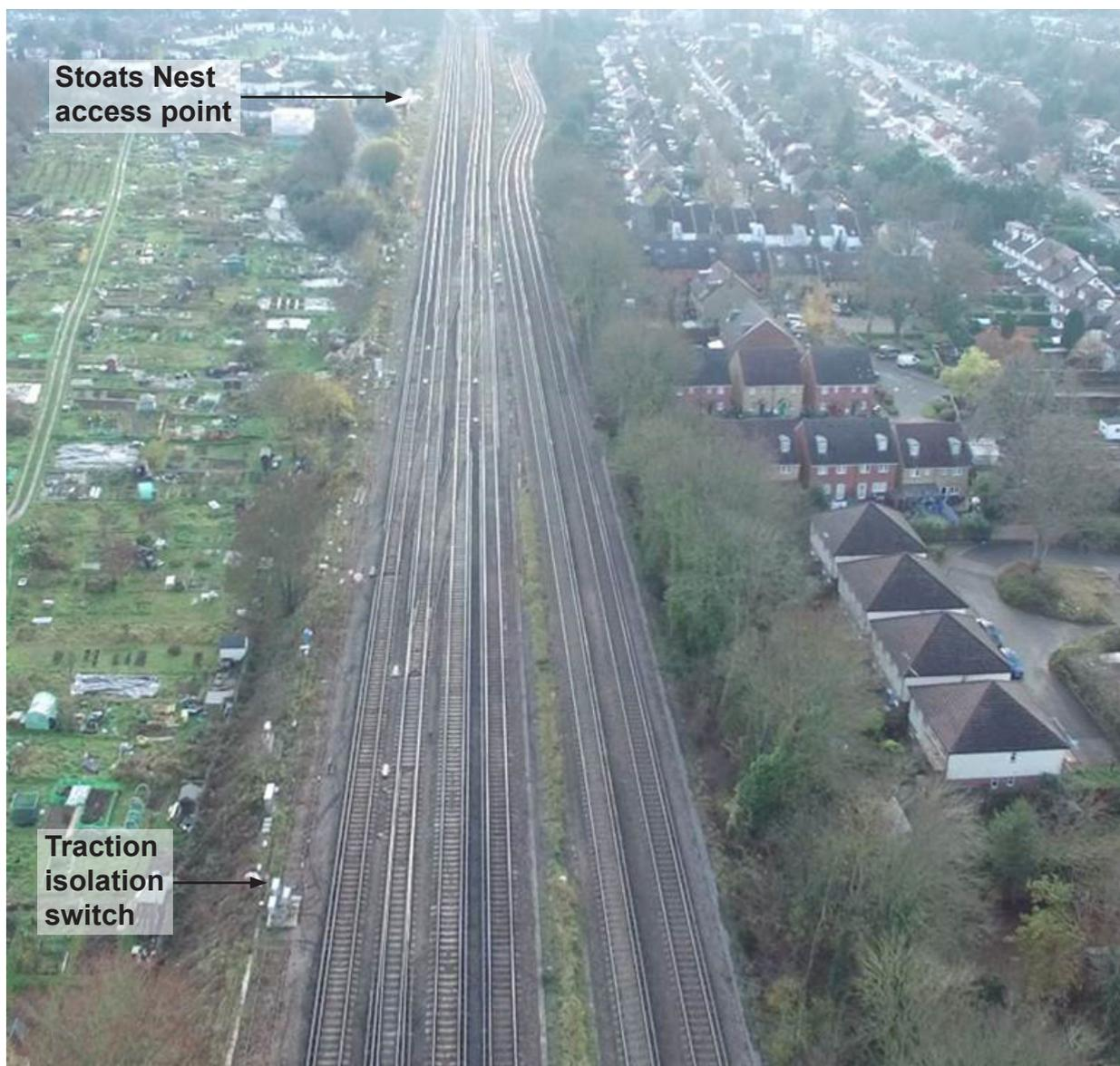
Figure 13: Image showing the location of the traction isolation equipment and Stoats Nest Road access point
