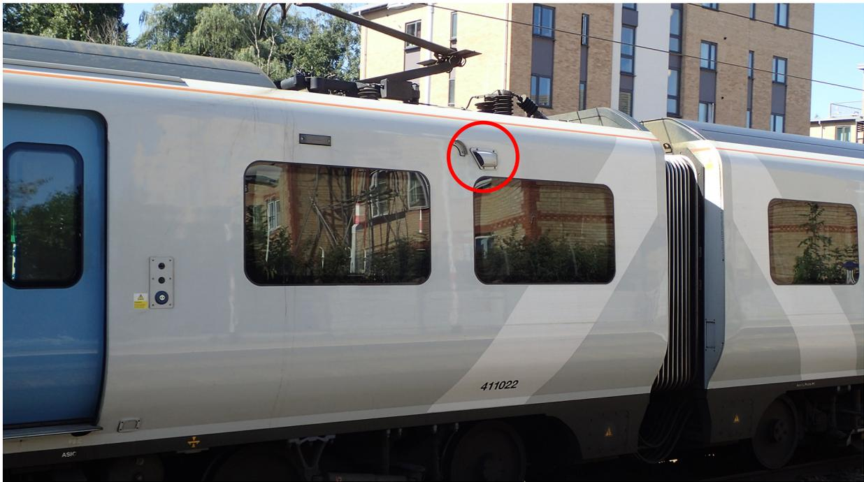
Figure 5: Exterior mounted CCTV camera (circled) on a class 700 coach
