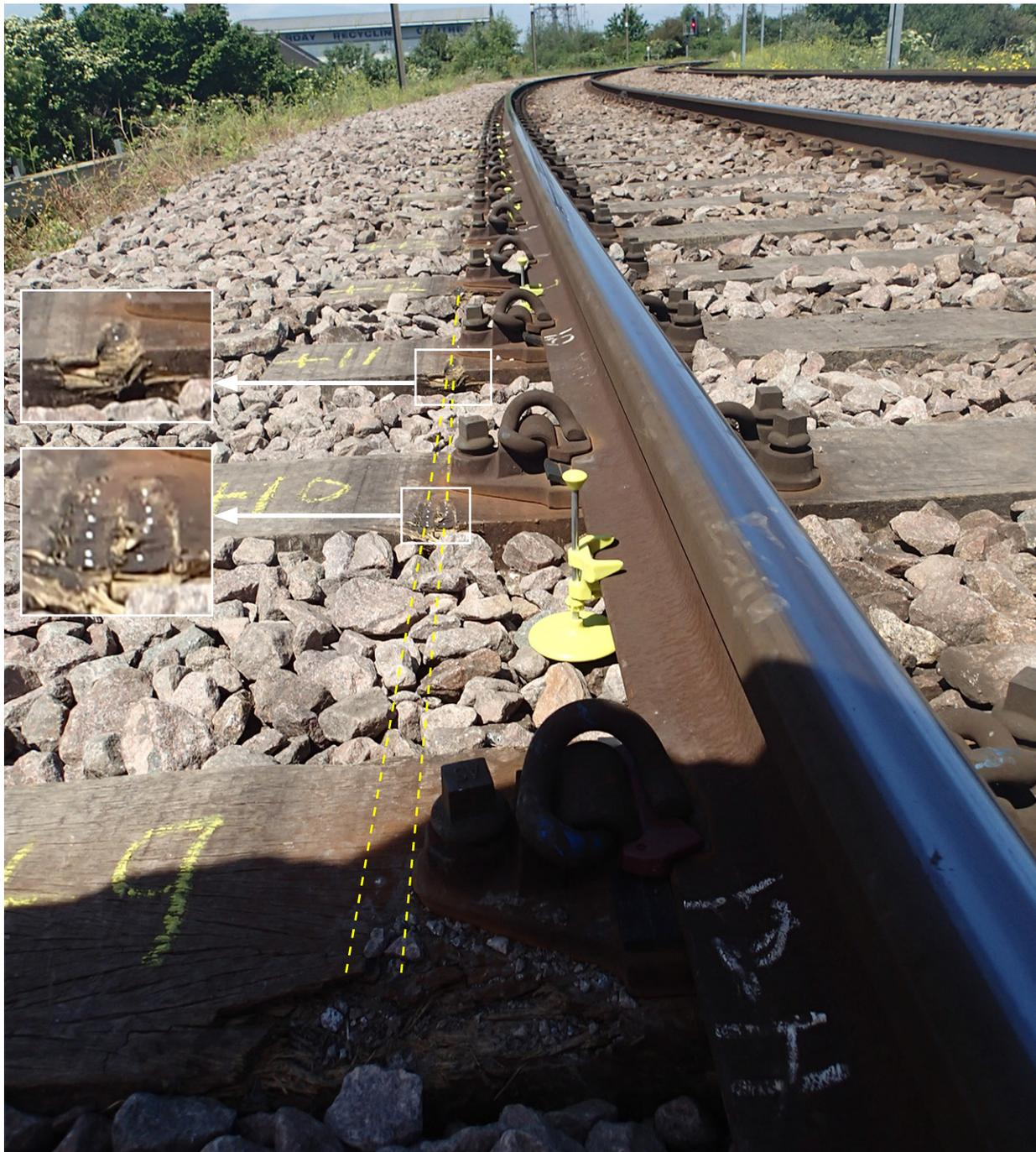
Figure 7: Marks showing evidence of derailed wheel flange running on the left-hand railhead, rail fasteners and sleeper ends (all photographs 23 May 2019, except as labelled)
