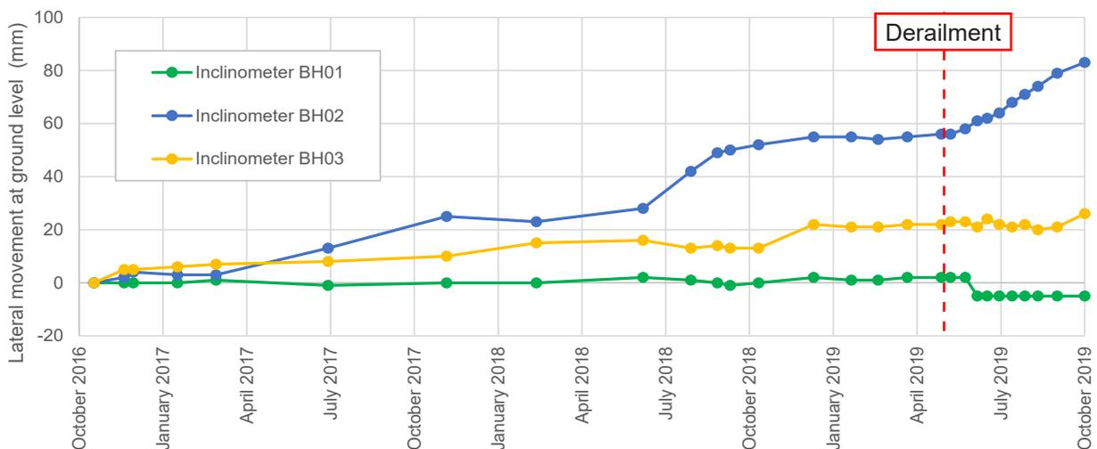
Figure 15: Lateral embankment movements measured at ground level by the inclinometers installed in the down-side slope (BH01) and the up-side slope (BH02 and BH03). Aerial image shows the location of the inclinometers.
