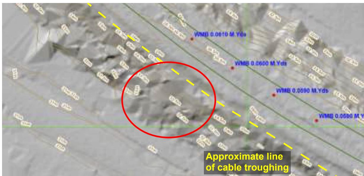
Figure 16: LiDAR survey of the embankment on Mitre Bridge Curve highlighting the flattened area on the up-side slope close to 0 miles 27 chains (image courtesy Network Rail)
