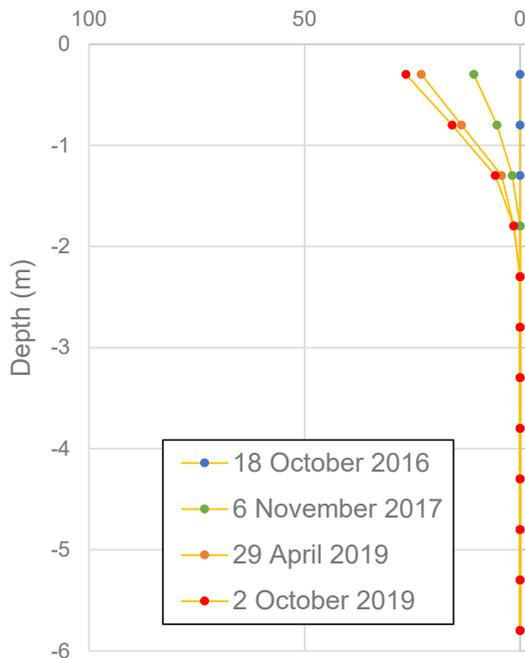
Ground movement at Inclinator BH02 (mm)
