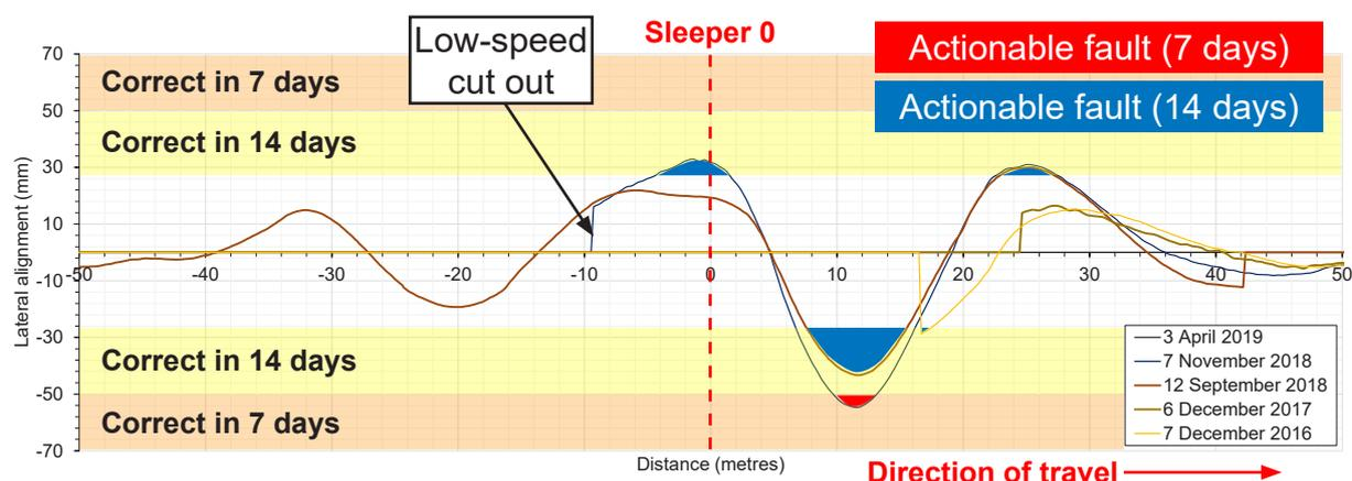
Figure 8: Lateral track alignment recorded on various track geometry measurement train runs prior to the derailment. Locations where low-speed cut out resulted in data loss are highlighted. On 3 April 2019 no lateral track geometry measurement data was recorded in the vicinity of the designated point of derailment, identified as 'Sleeper 0'.
