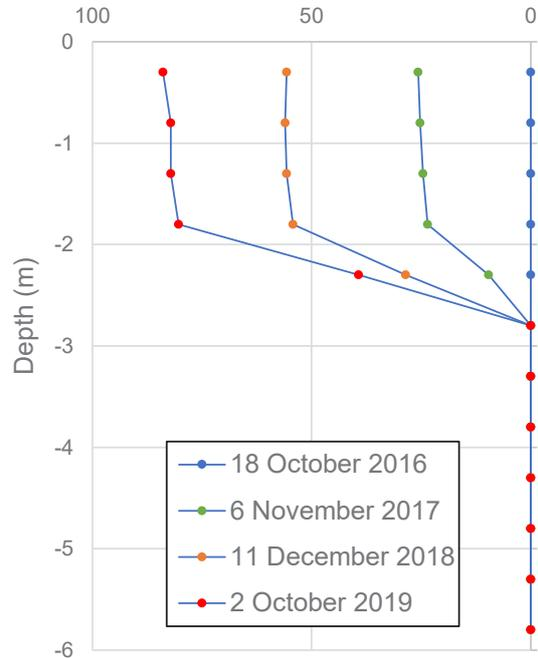
Figure 14: Cross-section of Mitre Bridge Curve embankment showing illustrative slip surface and simplified ground movement. Graphs show how the lateral movement measured at inclinometers BH02 and BH03 varied with borehole depth.
