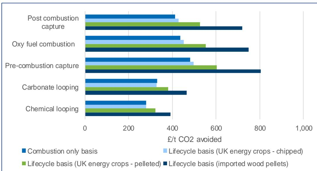
**Figure 3.6 Influence of biomass price on cost of carbon avoided on combustion only basis**
