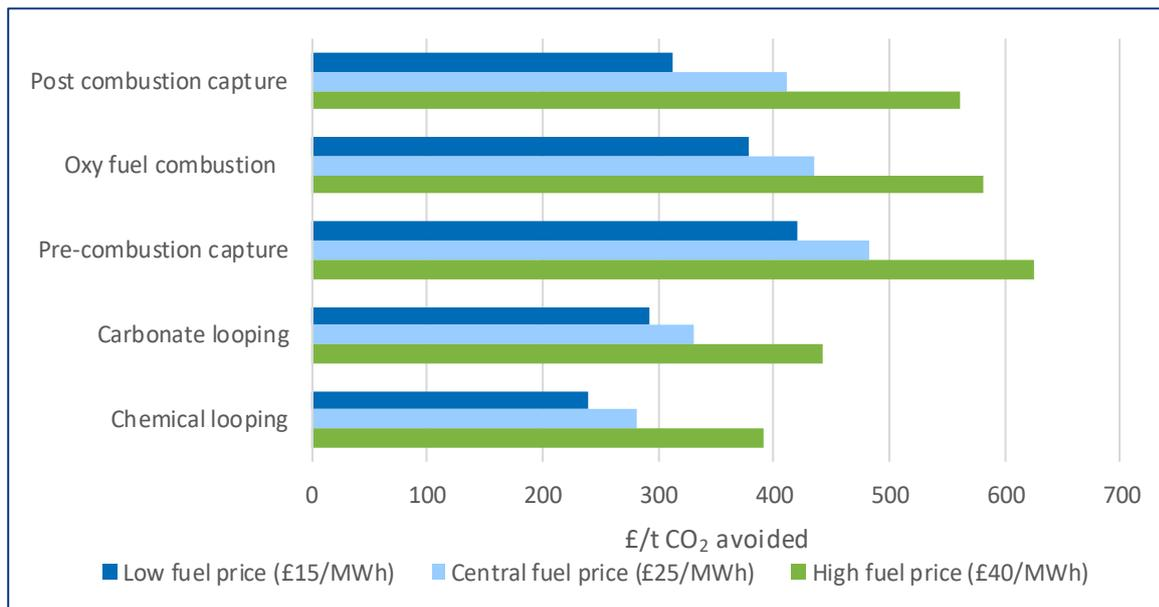
**Figure 3.7 Influence of biomass price on cost of carbon avoided on lifecycle basis (pelleted UK energy crops)**
