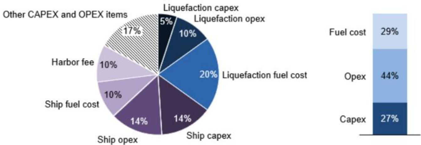
**Figure 30: Unit cost of CO2 transport for transporting 1 MtCO2/year over a distance of 600 km and timeframe of 20 yr**
