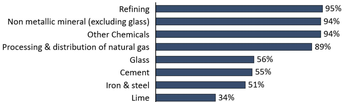
The technical decarbonisation potential of H2 fuel switching in the sectors considered in this analysis is a 72% reduction in emissions.
