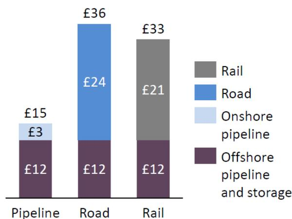
**Figure 21: Carbon intensity of transport to port terminal (CO<sub>2</sub> emitted per CO<sub>2</sub> transported)**
