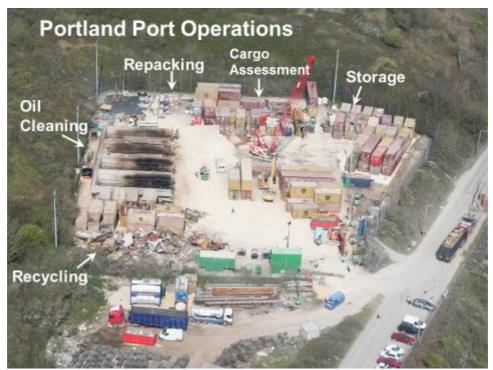
Figure 2 - The bunded areas as set up during the NAPOLI operations at Portland Port in 2007 is an example of good practice.
