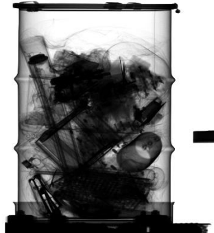
Figure 6: An X-ray of a typical 200 Litre drum
