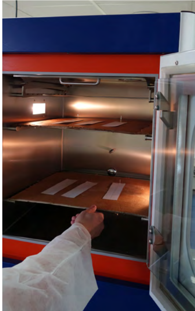
Loading the Ninhydrin cabinet for testing
