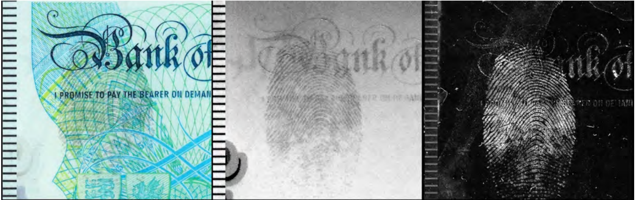
A fingerprint visualised with Powder Suspension, as viewed under white light (left), via reflected infrared (middle) and from a gelatin lift scan (right)
