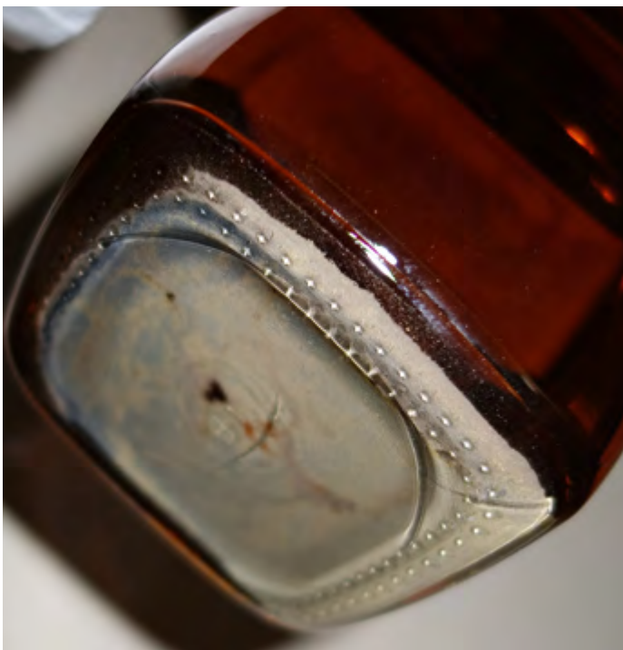
A failed alternative to Synperonic N has not kept the silver in solution and this has precipitated at the bottom of the bottle
