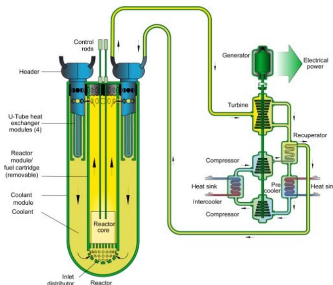
**Figure 17: Generic Gen. IV Lead-cooled Fast Reactor**
