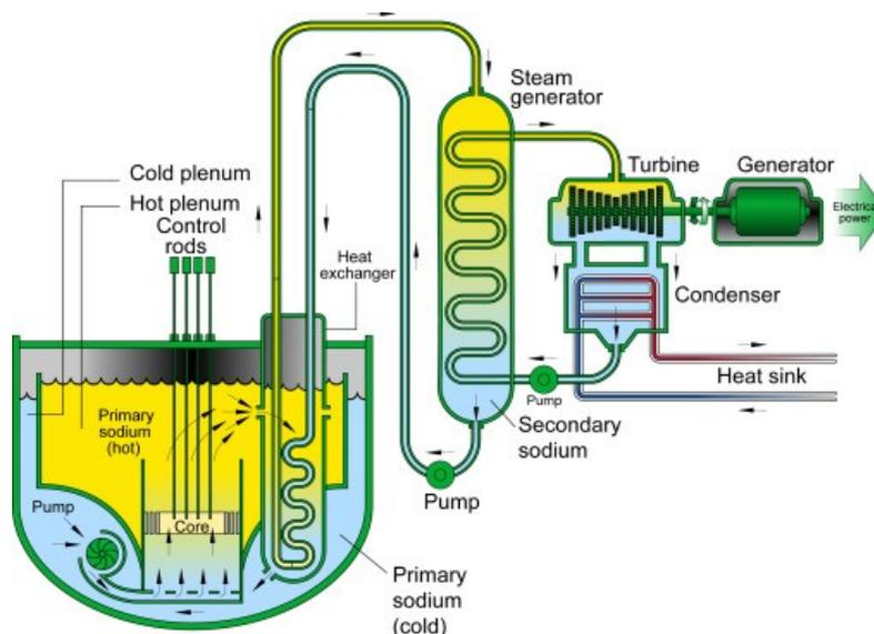
**Figure 11: Generic Gen. IV (pool-type), Sodium-cooled Fast Reactor**
