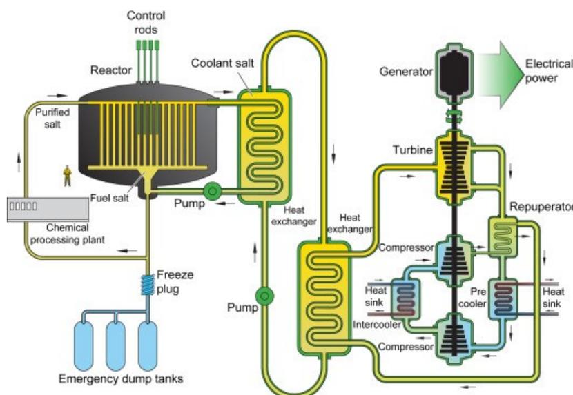
**Figure 23: Generic Gen. IV Molten Salt-fuelled Reactor**
