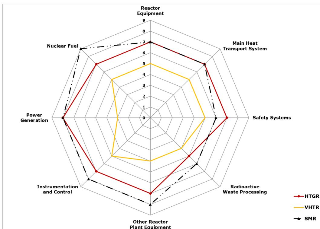
Figure 9: Comparison of HTGR, VHTR and SMR TRLs
