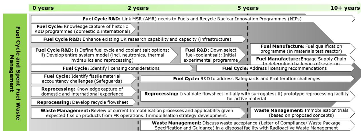
Figure 26: Roadmap of MSR Fuel Cycle and Spent Fuel Waste Management needs
