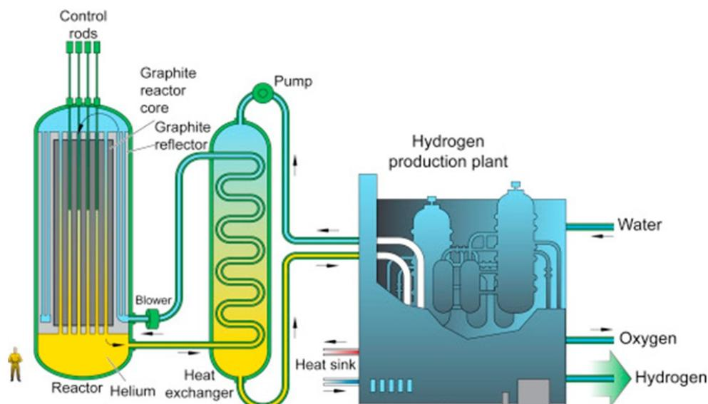
**Figure 2: Generic Gas-cooled Reactor (Prismatic Core) with coupled H<sub>2</sub> production facility**
