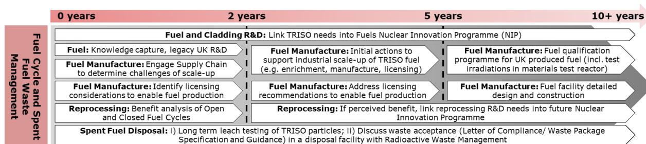
**Figure 5: Roadmap of HTGR Fuel Cycle and Spent Fuel Waste Management needs**
