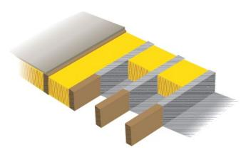
Quilted insulation supported by netting stapled to joist
