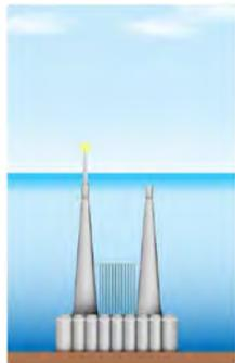
Option 5 would involve removing the steel transitions. Shallow cut zones would be cleared and leg internals above this removed.
