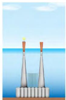
Option 9 would involve topside removal only, leaving the four steel transitions in place.
