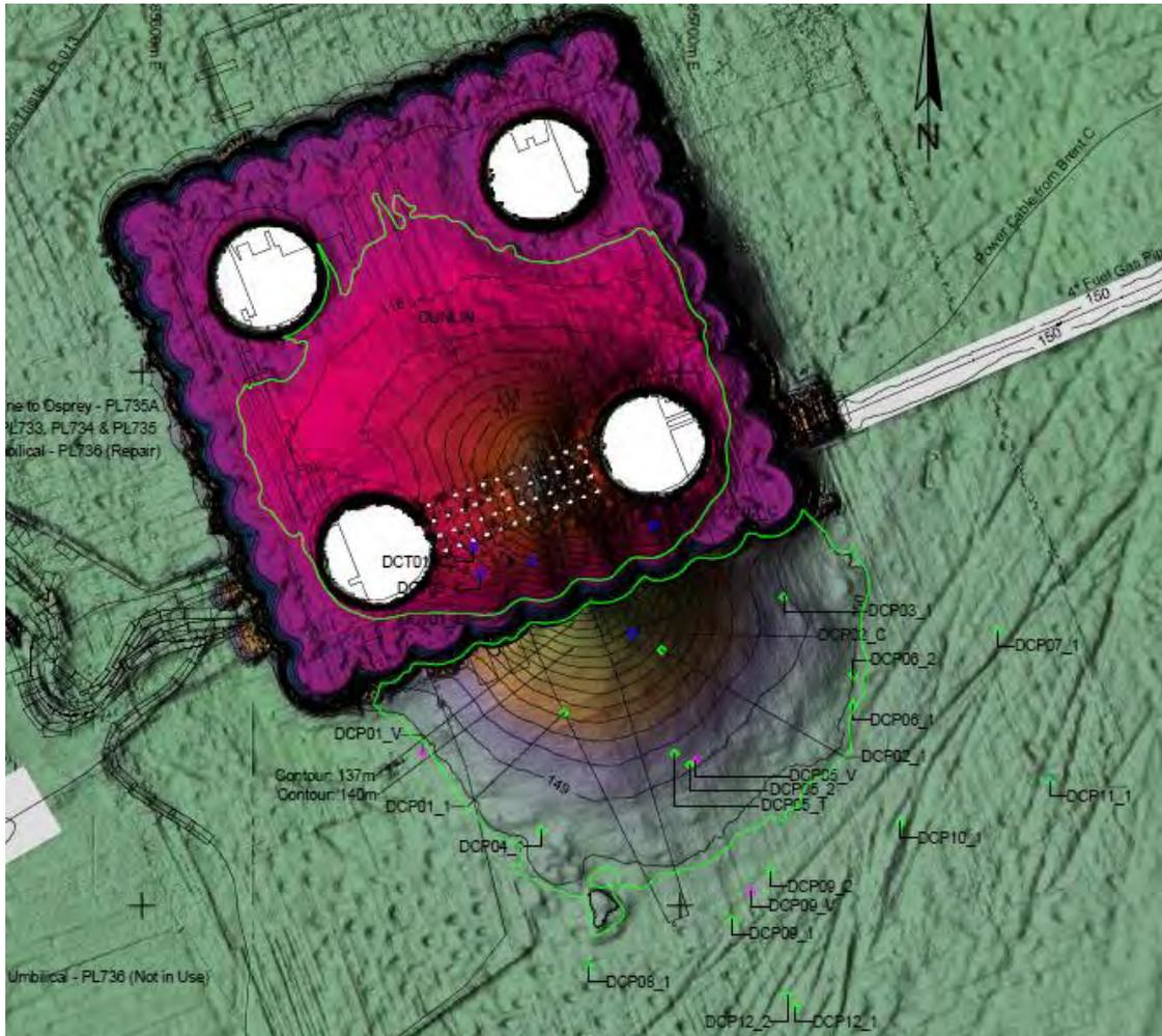
**Figure 2.13 Drill cuttings profile at the Dunlin Alpha platform**
