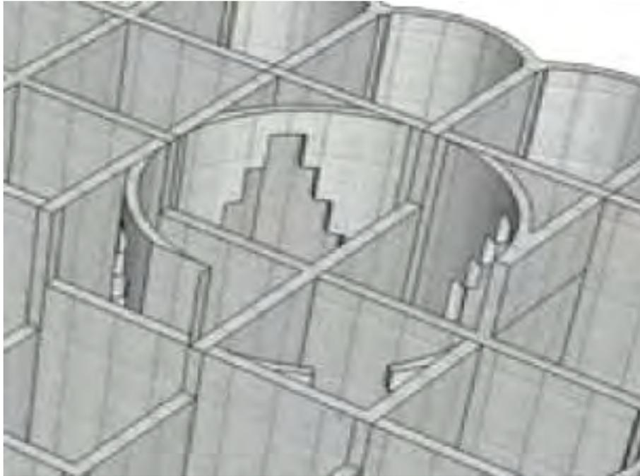
**Figure 2.7 Triangle cells below CGBS leg structure**
