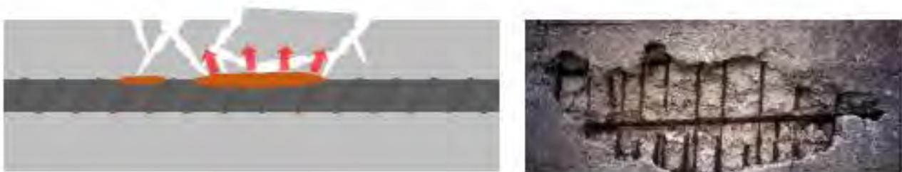
**Figure 5.1 Spalling of reinforced concrete**
