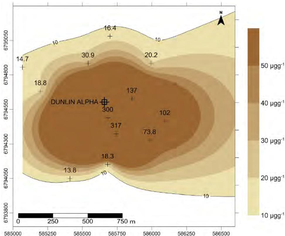
**Figure 5.8 Spatial distribution of surface sediment total hydrocarbon concentrations showing 50 ppm hydrocarbon content boundary**
