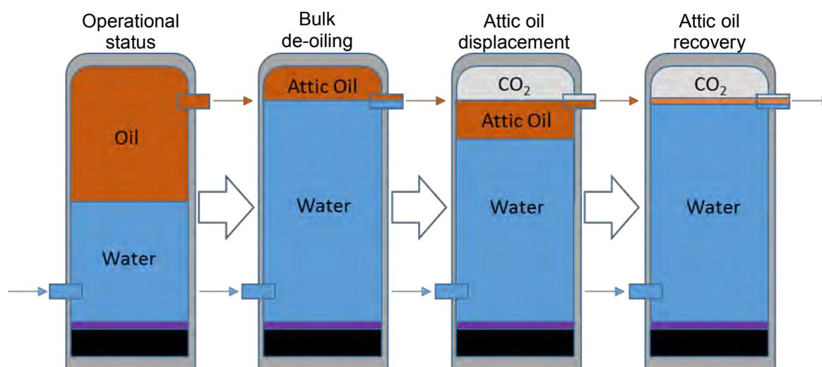
Figure 2.9 Overview of the Attic Oil Recovery Project
