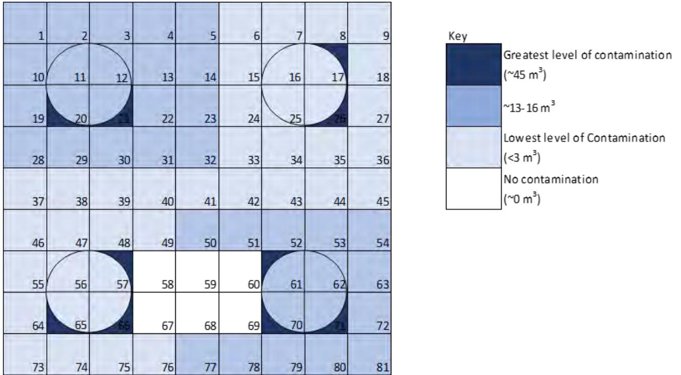
**Figure 2.12** Distribution of hydrocarbon contamination with the CGBS storage cells
