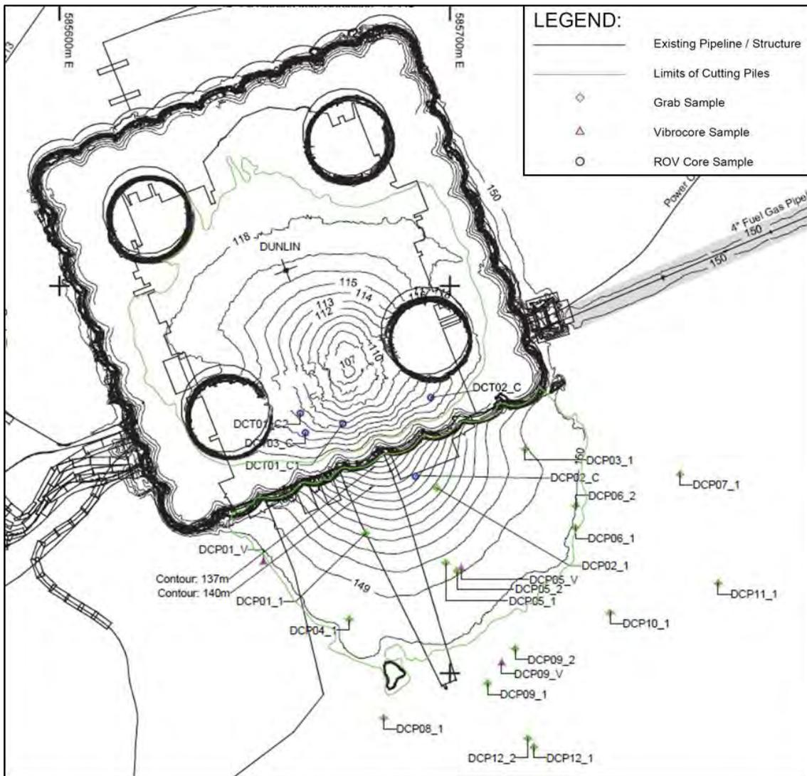
**Figure 4.4 Dunlin Alpha cuttings pile sample locations**
