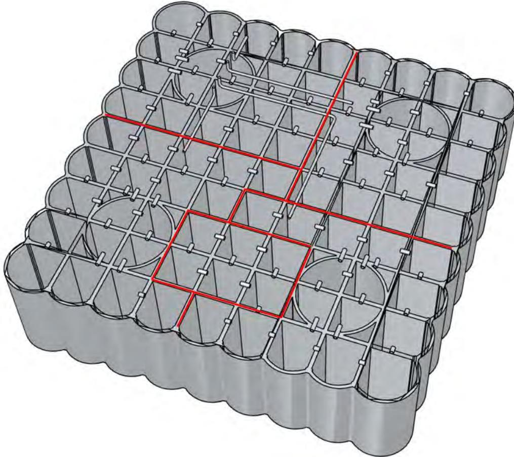
**Figure 2.5 Cells in the CGBS (cutaway view)**
