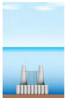
Option 6 would involve removing the steel transitions and upper concrete leg sections. Shallow and IMO compliant cut zones would be cleared and leg internals above these removed.
