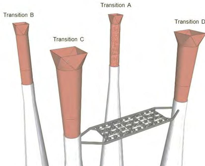
**Figure 2.4 Transitions at the tops of the concrete legs (topsides and conductors not shown)**
