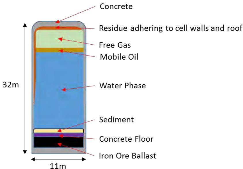
**Figure 2.10 Representative schematic of a cell and residual contents (not to scale)**
