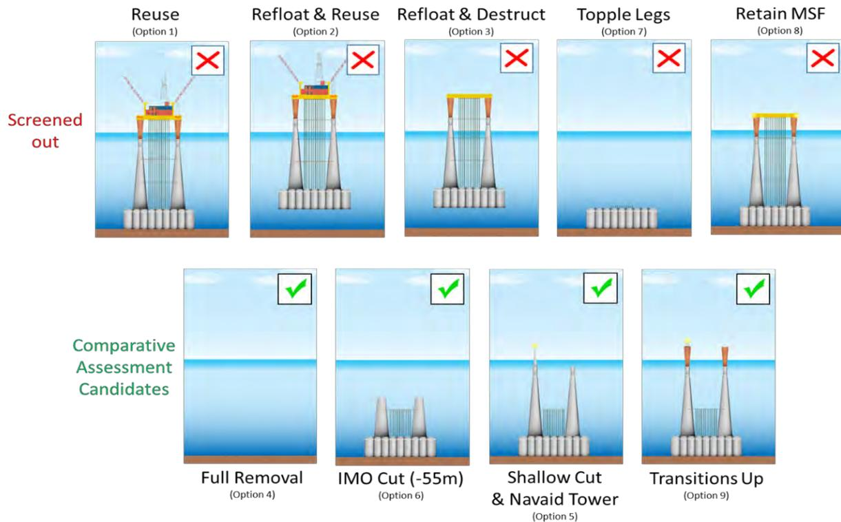
**Figure 2.14 Option screening for the substructure**
