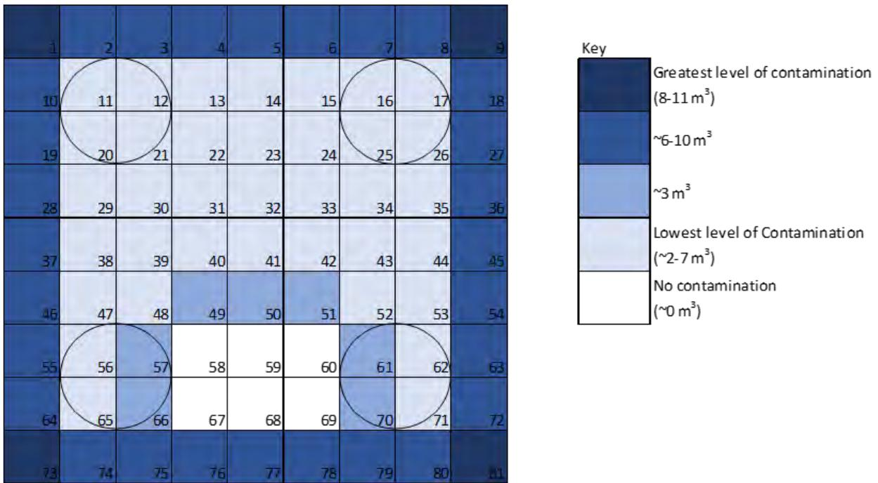
**Figure A 3 Distribution of wall residue (wax) contamination within the storage cells**
