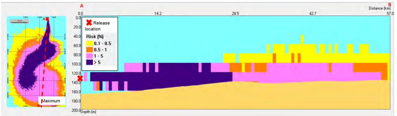
Figure D2 Water column risk – section view of maximum extent
