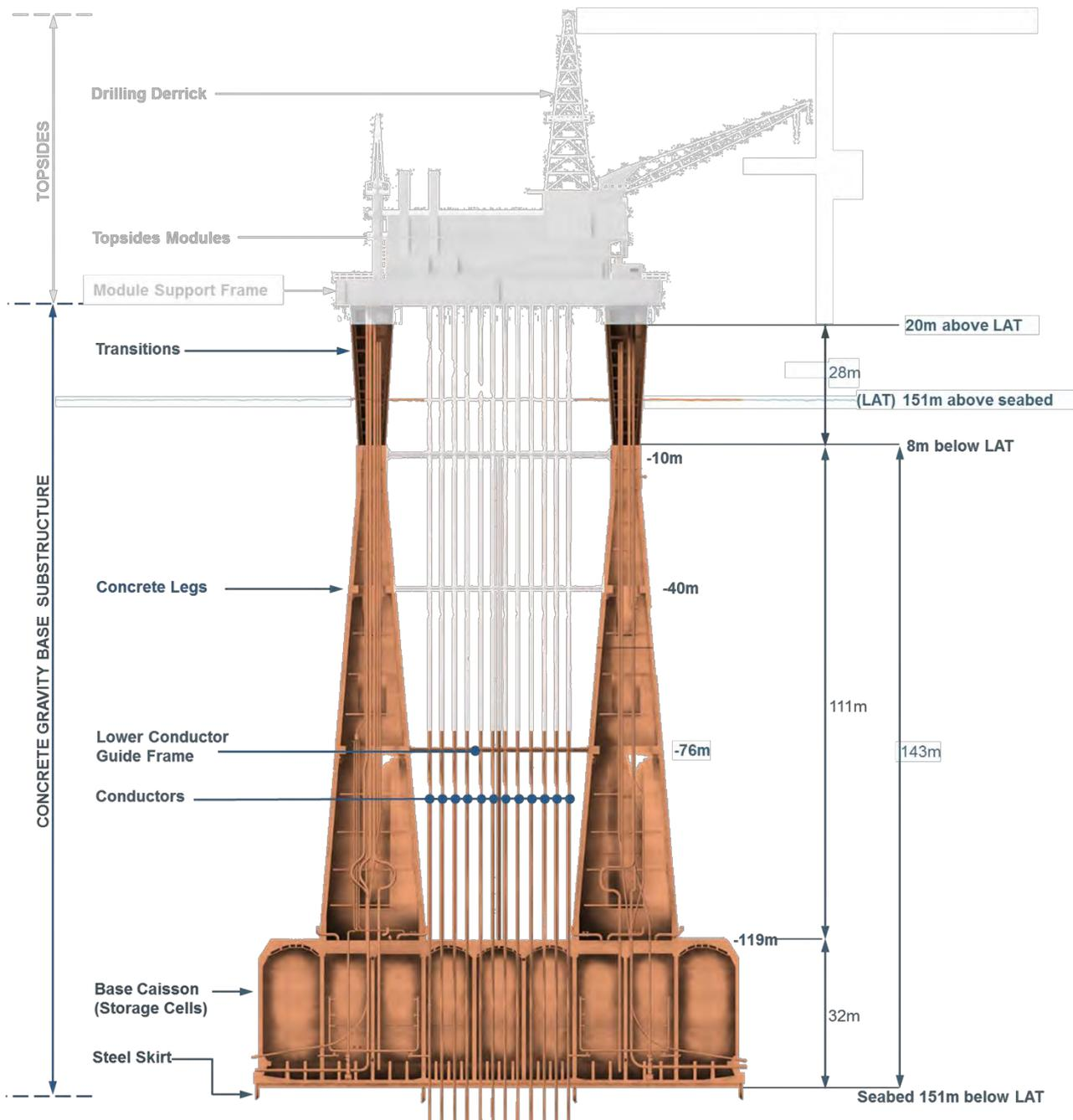
**Figure ii Dunlin Alpha concrete gravity base substructure**
