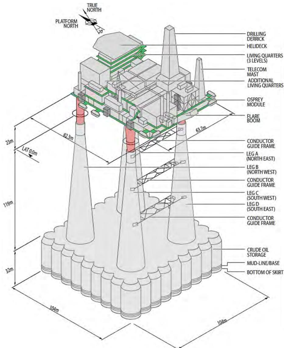
**Figure 2.1 Schematic of the Dunlin Alpha installation**
