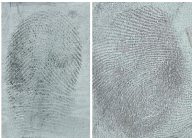
Fingermarks visualised by the new DGME-based PD (left) and the Synperonic N PD formulation (right)
